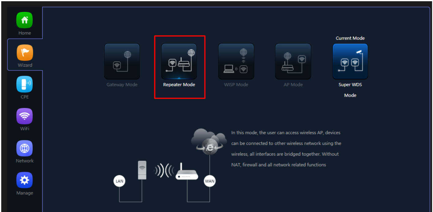
Fig 2.2.1 Repeater mode of AirONE AIR-CPE10K+
