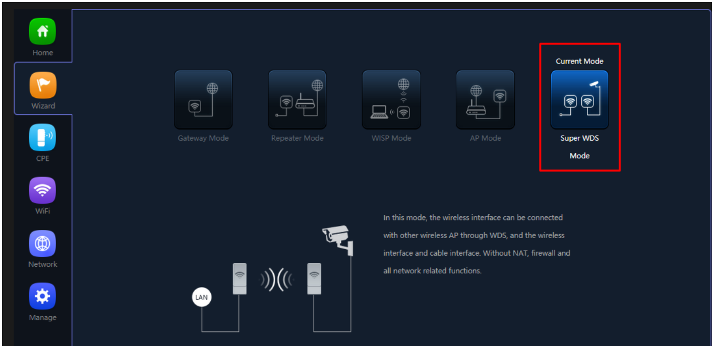
Fig 2.5.1 Super WDS mode of AirONE AIR-CPE10K+
