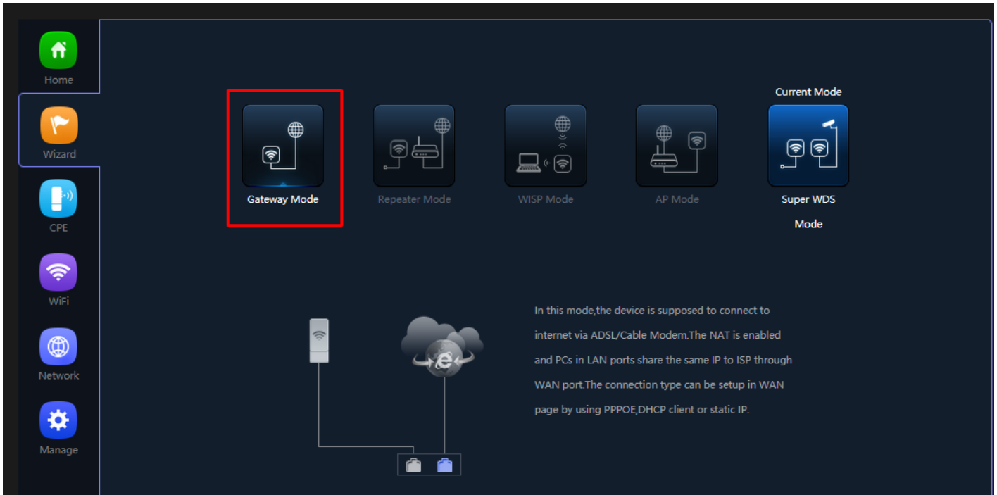
Fig 2.1.1 Gateway mode of AirONE AIR-CPE10K+
