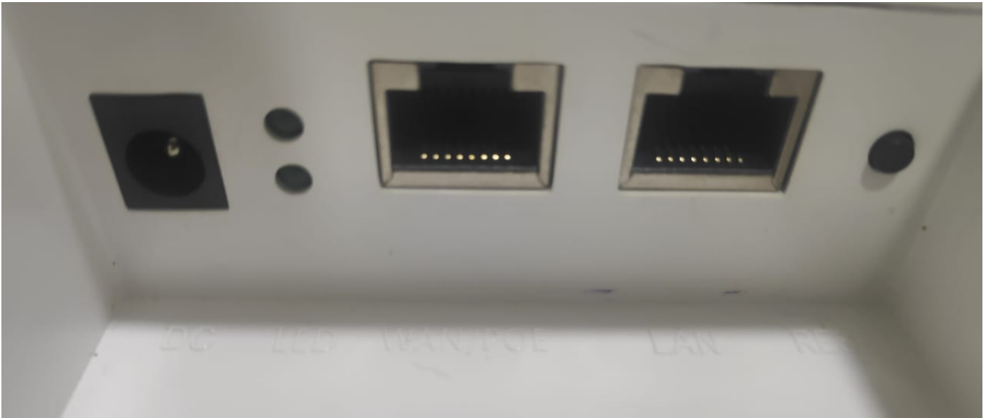
Fig 1. Physical port on AirONE AP1800AX-HD
