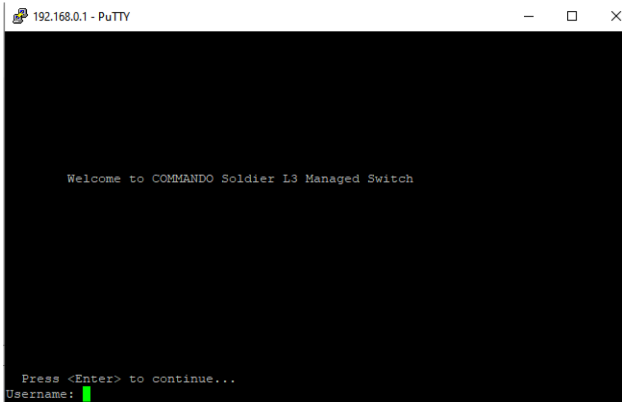
Fig-13. COMMANDO Series E3000 Switch CLI access via telnet
