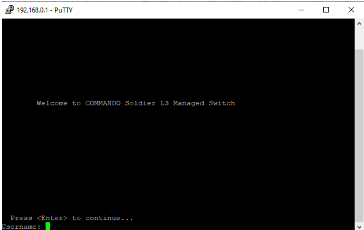
Fig-3. COMMANDO Series E3000 Switch CLI access via console port
