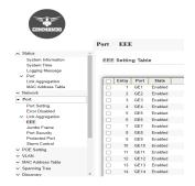
Fig 4.4.4 Port EEE Setting Table after Enabled Port page
