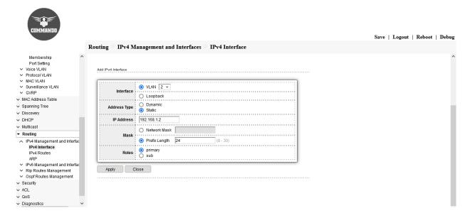
Fig 11.3.4 Add Static VLAN IP address with subnet mask Page
