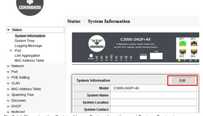
Fig 2.1.1 Changing the System Name, System Location and System Contact
