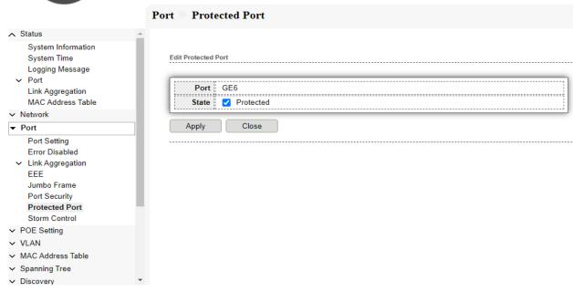
Fig 4.7.3 Enable GE6 port for Protected Port configuration page
