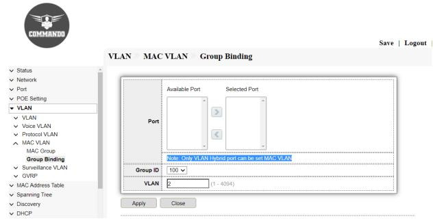
Fig 5.4.5 Blank Group binding for hybrid ports page
