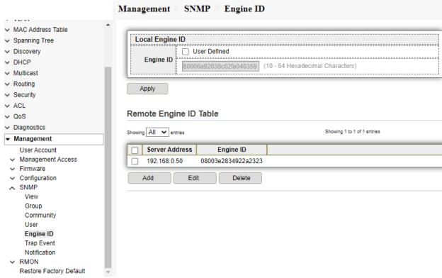
Fig 16.5.15 SNMP Add Remote Engine ID page
