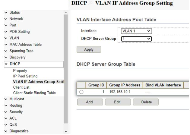
Fig 9.3.2 DHCP Binding VLAN Interface to DHCP server group IP address page.
