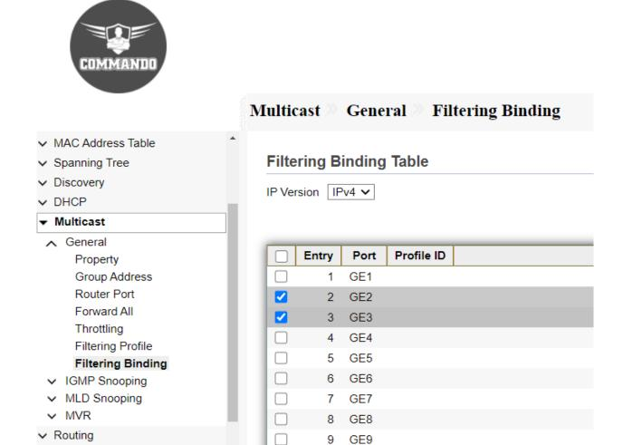
Fig 10.1.17 Multicast filtering Binding Port selection page
