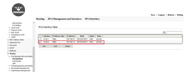
Fig 11.3.5 Assign IP address to created VLAN Page
