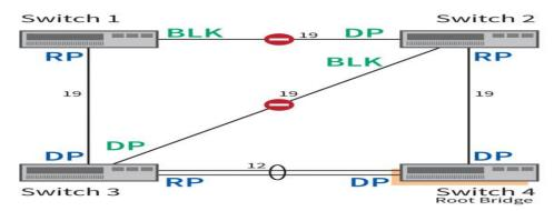
Fig 7.1.1 Spanning Tree enabled network Changed topology.
