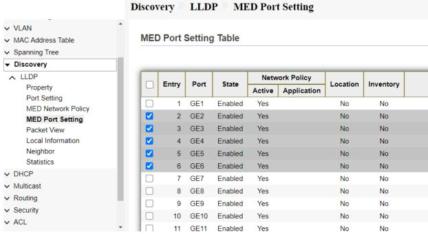
Fig 8.4.2 LLDP MED port setting for ports page
