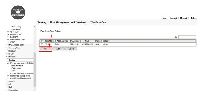
Fig 11.4.2 Add IP address for VLAN Page
