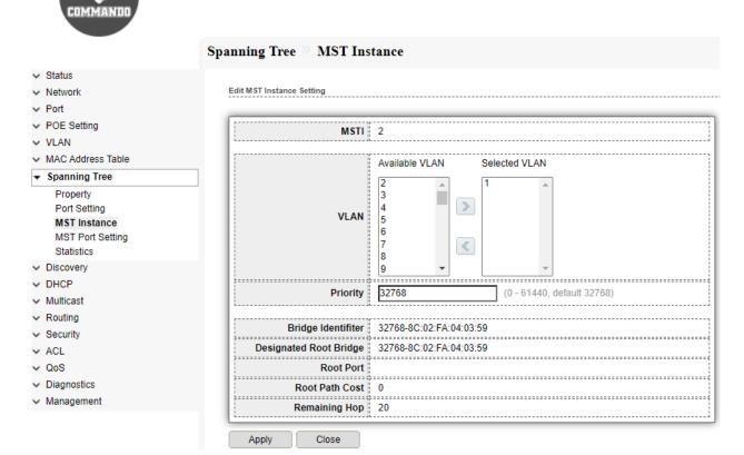
Fig 7.3.3 Spanning tree MST interface setting page
