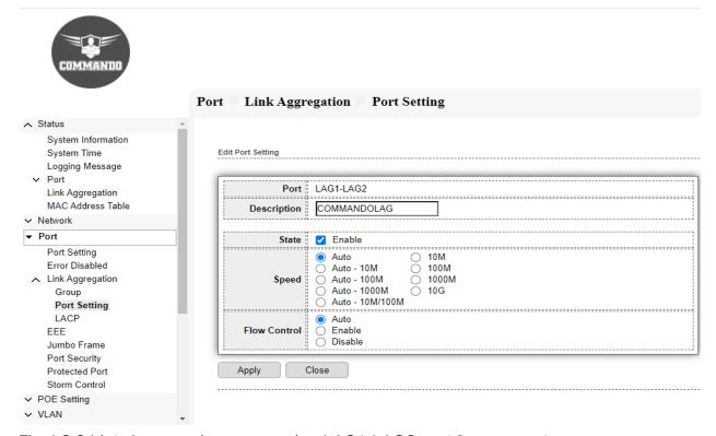
Fig 4.3.9 Link Aggregation port setting LAG1-LAG2 and flow control page
