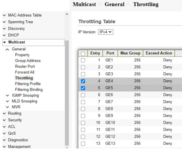
Fig 10.1.11 Multicast Selecting port for throttling page
