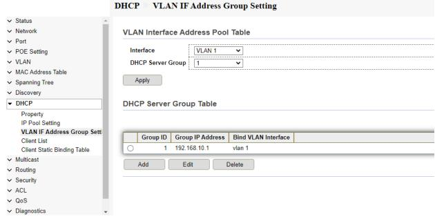
Fig 9.3.3 DHCP Binding VLAN Interface to DHCP server group
