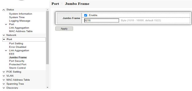
Fig 4.5.2 Jumbo Frame Enable for 9216 bytes page
