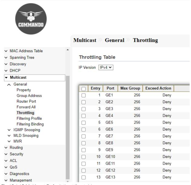
Fig 10.1.10 Multicast Default throttling table page
