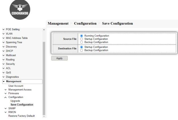
Fig 16.4.4 Save running Configuration to Startup Configuration page
