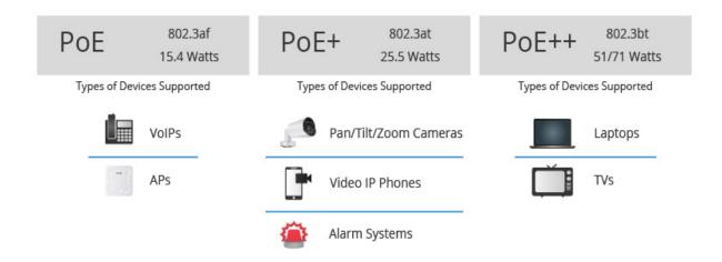
Fig 17.1 C3000 Series PoE/PoE+/Ultra PoE++ Switches Concept
