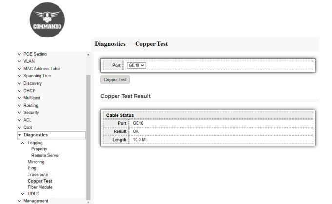
Fig 15.4.2 Diagnostic Copper Test Result page
