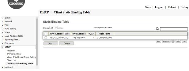
Fig 9.5.3 DHCP Client Static Binding Table page.
