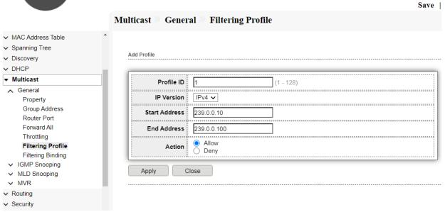
Fig 10.1.14 Multicast Add filtering profile page
