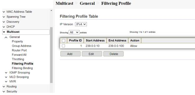
Fig 10.1.15 Multicast filtering profile table page
