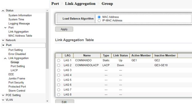
Fig 4.3.6 Link Aggregation group configuration page
