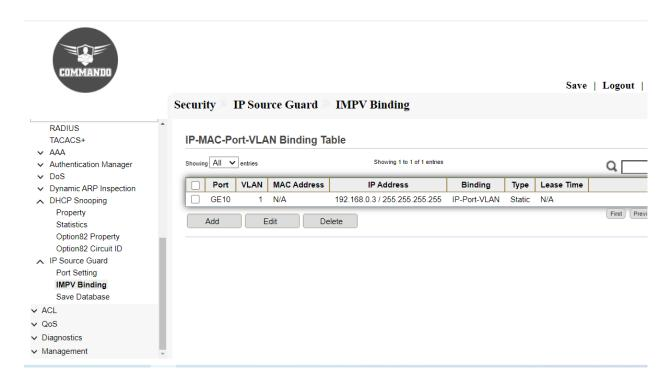
Fig 12.9.8 IP Source Guard IP-MAC-Port-VLAN Binding Table page
