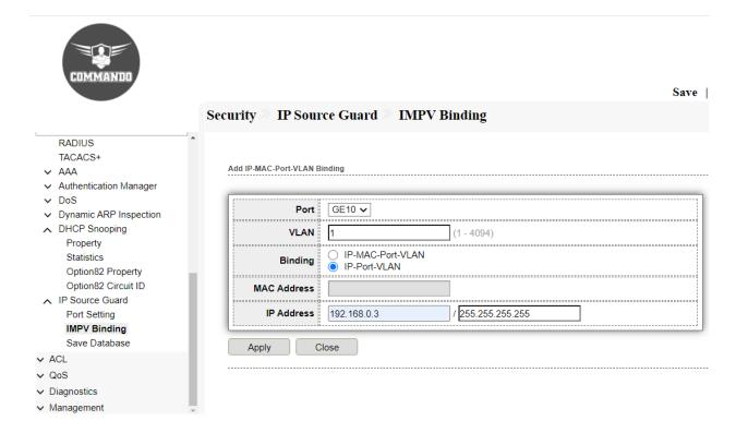
Fig 12.9.7 Add IP Source Guard IP-MAC-Port-VLAN Binding page
