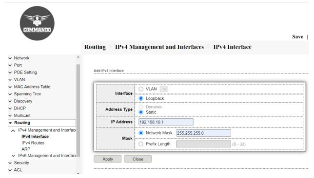
Fig 11.1.3 Creating IPv4 loopback interface configuration page
