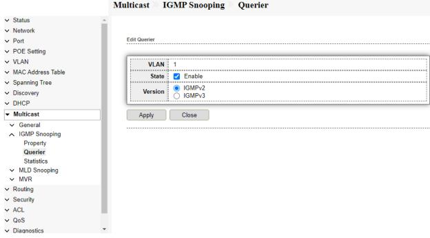
Fig 10.2.6 IGMP snooping Selecting VLAN Querier page
