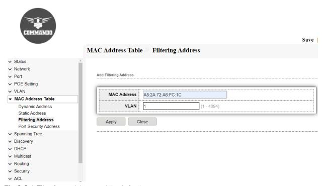
Fig 6.3.1 Filtering address table default page
