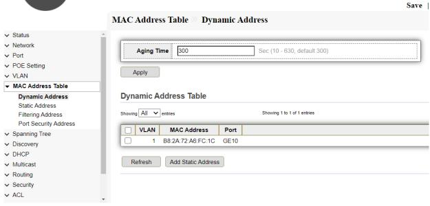
Fig 6.1.2 Add Static address from Dynamic MAC address table page
