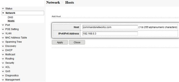
Fig 3.2.2 Add DNS Host and IP address configuration page
