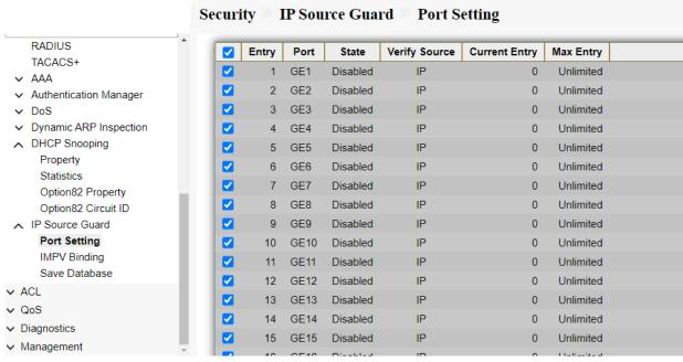
Fig 12.9.3 IP source guard Selecting Ports for Setting page
