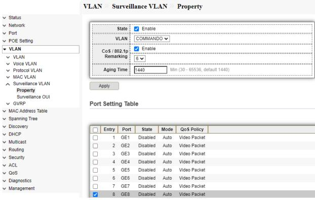
Fig 5.5.2 Surveillance VLAN port setting page for selected GE4 port
