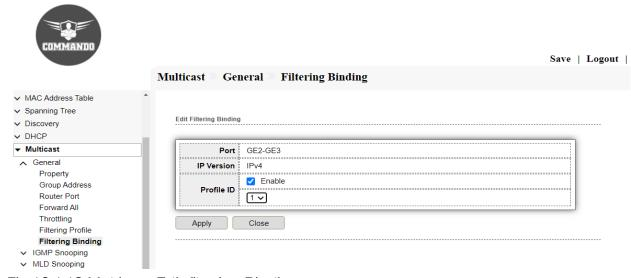
Fig 10.1.18 Multicast Edit filtering Binding page
