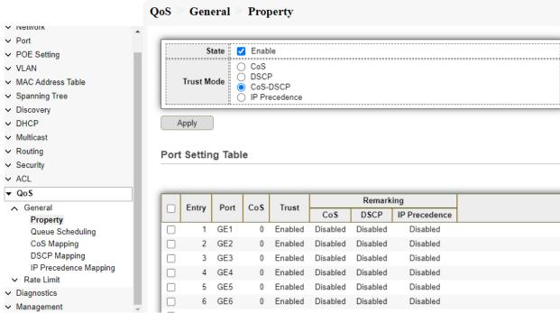
Fig 14.1.2 Enable QoS on Switch page
