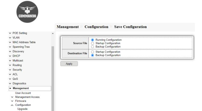
Fig 16.4.5 Save running Configuration to Backup Configuration page
