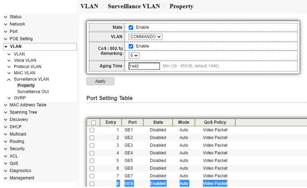
Fig 5.5.4 Surveillance VLAN Port setting table GE8 port enabled for Video packet
