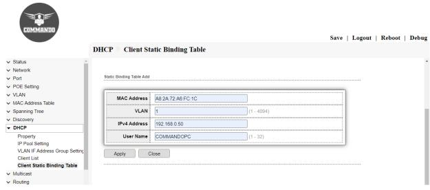
Fig 9.5.2 DHCP Client add static binding page.
