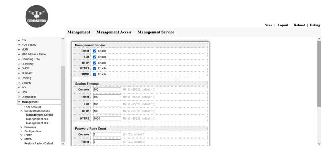
Fig-8. COMMANDO C3000 Switch Management Access service.
