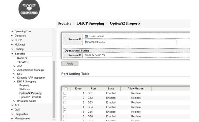
Fig 12.8.9 DHCP Snooping Option82 Edit Port Setting Table page after Enabling Ports page
