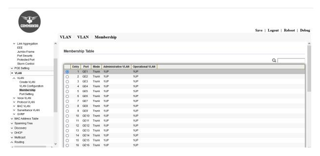
Fig 11.3.6 Selecting Interface to assign new VLAN membership page
