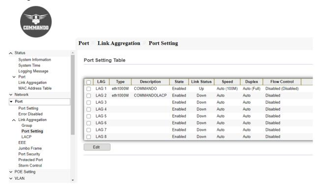
Fig 4.3.7 Link Aggregation port setting table page
