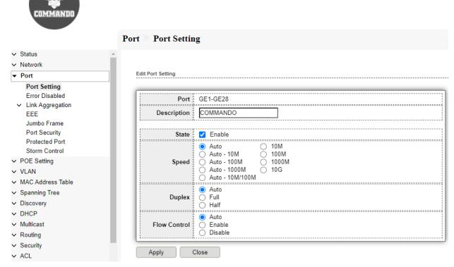
Fig 4.1.3 Port setting multiple ports Description, status, speed, duplex, flow control selection page.
