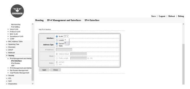
Fig 11.4.3 Selecting VLAN for providing IP address Page
