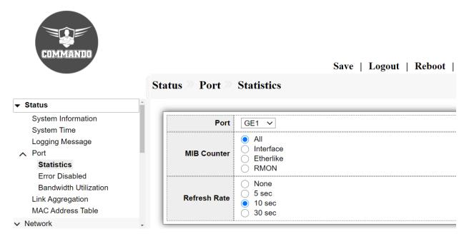
Fig 2.4.1 Port selection for MIB Counter Statistics
