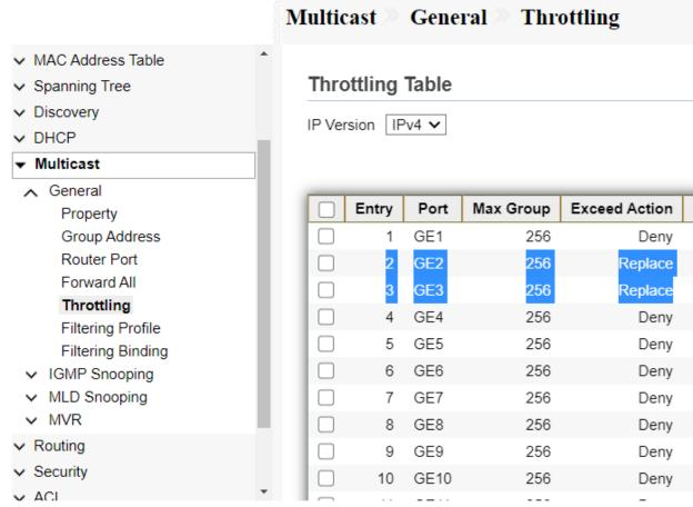
Fig 10.1.13 Multicast throttling Table page
