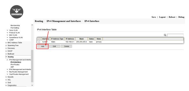
Fig 11.3.2 Add IP address for VLAN Page
