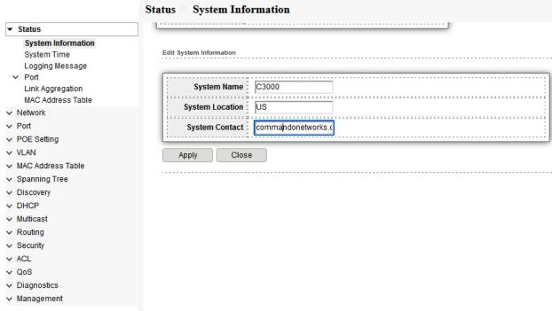
Fig 2.1.2 Changing System Name, System Location and System Contact
