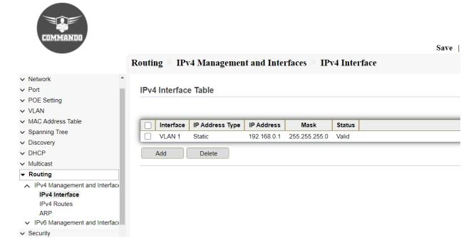
Fig 11.1.2 IPv4 interface configuration page
