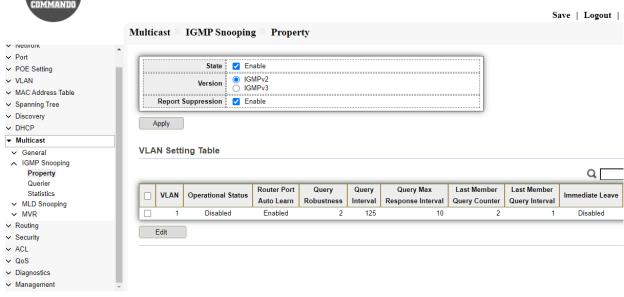
Fig 10.2.2 IGMP snooping property VLAN setting page
