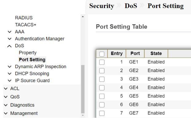
Fig 12.5.5 DoS Port Setting Table after enabled ports page
