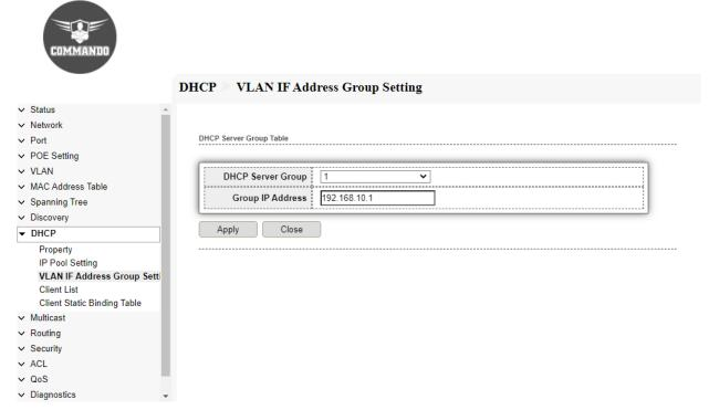
Fig 9.3.1 DHCP VLAN Interface address pool and Server group table page.
