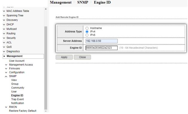
Fig 16.5.14 SNMP Add Remote Engine ID page
