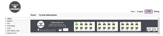
Fig 1.3.5 Reboot button on Web GUI
