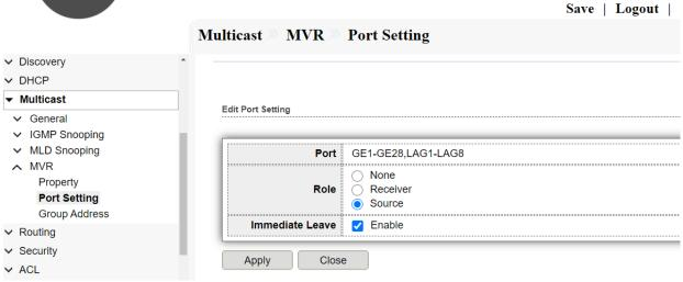
Fig 10.4.5 Multicast MVR Edit port setting page
