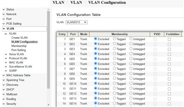
Fig 5.1.7 VLAN Selection tap on VLAN configuration table page
