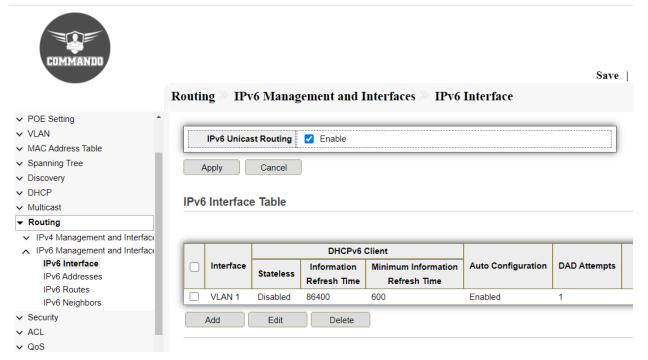
Fig 11.2.2 Enable IPv6 Unicast Routing page
