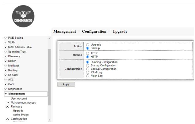
Fig 16.4.2 Backup of Configuration from running configuration page
