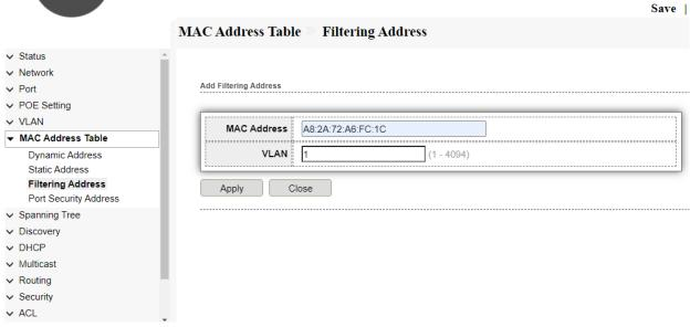
Fig 6.3.2 Add Filtering MAC address to Specified VLAN page
