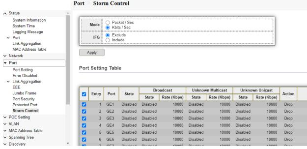
Fig 4.8.2 Storm control Selecting port setting page
