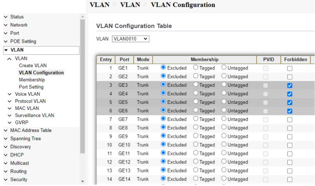
Fig 5.1.8 VLAN configuration for Ports selection page
