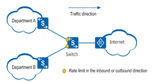
Fig 14.2.1 Rate Limiting concept
