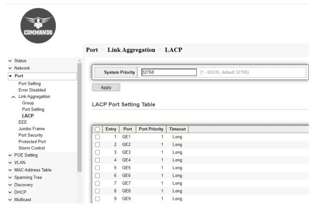
Fig 4.3.6 Link Aggregation LACP Port Setting Table page
