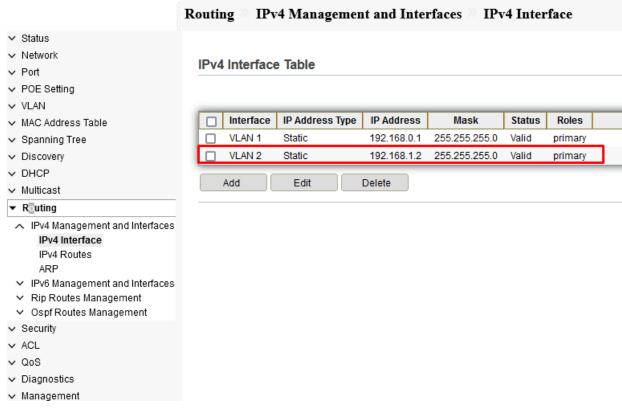
Fig 11.1.7 IPv4 address for VLAN 2 page
