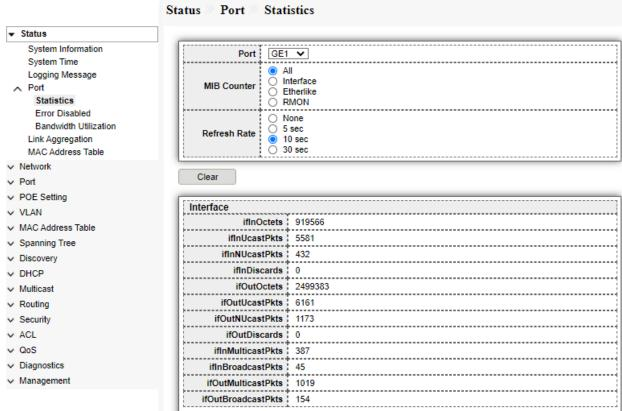
Fig 2.4.2 Gigabit Ethernet 5 port selection for MIB Counter Statistics
