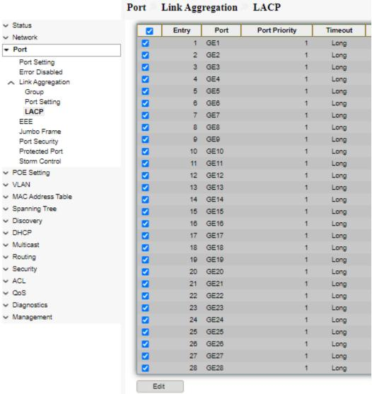
Fig 4.3.7 Link Aggregation LACP Port Setting port selection page
