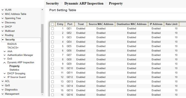
Fig 12.6.5 DAI Port Setting Table page after enabling ports page
