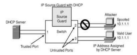
Fig 12.9.1 IP Source Guard concept
