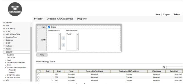
Fig 12.6.2 Dynamic ARP Inspection (DAI) port setting table page
