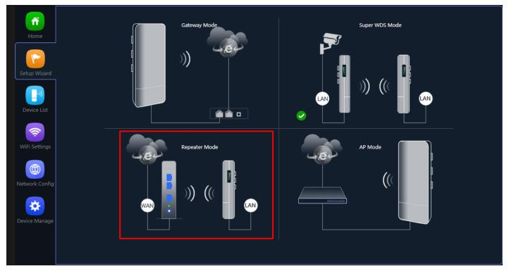
Fig 2.3.1 Repeater mode of AirONE AIR-CPE5K+
