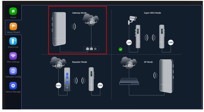
Fig 2.1.1 Gateway mode of AirONE AIR-CPE5K+
