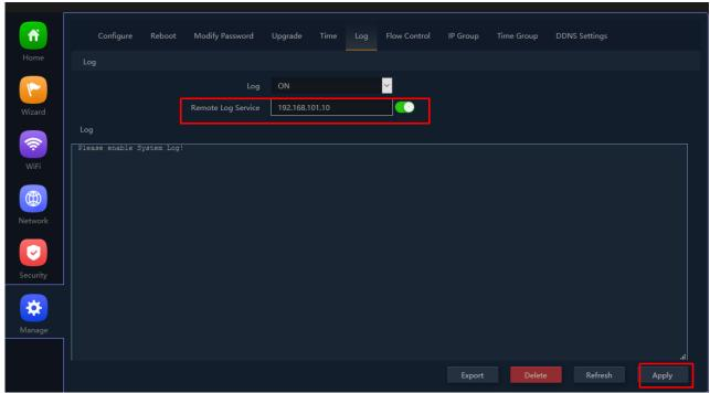
Fig 7.6.3 Remote Log service setting IP for AirONE AIR-CPE1K+
