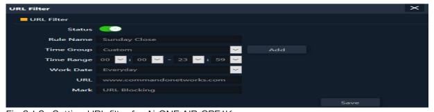
Fig 6.1.2 Setting URL filter for AirONE AIR-CPE1K+
