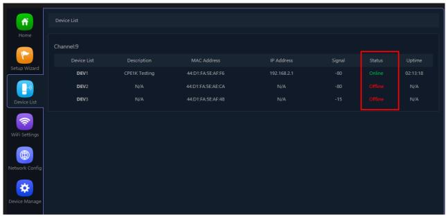
Fig 3.1.1 Device list of AirONE AIR-CPE1K+
