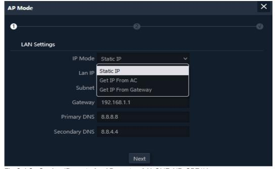
Fig 2.4.2 Setting IP mode for AP mode of AirONE AIR-CPE1K+
