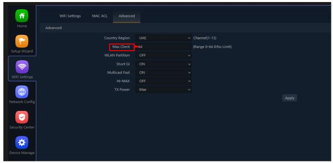
Fig 4.4.3 Max Client for AirONE AIR-CPE1K+
