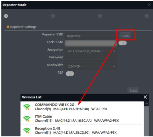
Fig 2.3.2 Selecting Repeater SSID of AirONE AIR-CPE1K+
