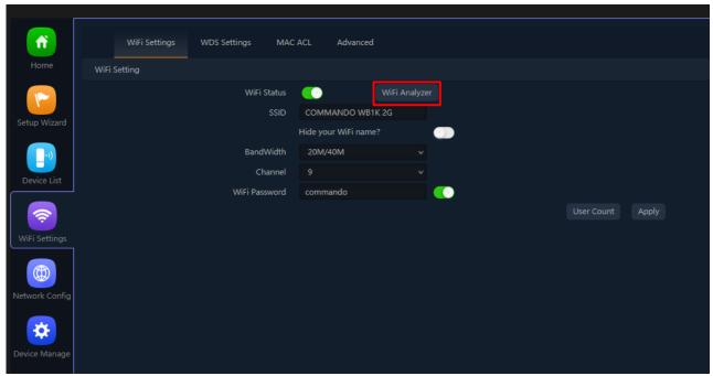
Fig 4.1.2 2G Wi-Fi Analyzer button of AirONE AIR-CPE1K+
