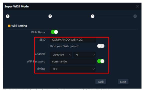
Fig 2.2.5 Wi-Fi Setting in Super WDS mode of AirONE AIR-CPE1K+
