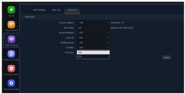
Fig 4.4.7 Selecting HI-MAX for AirONE AIR-CPE1K+
