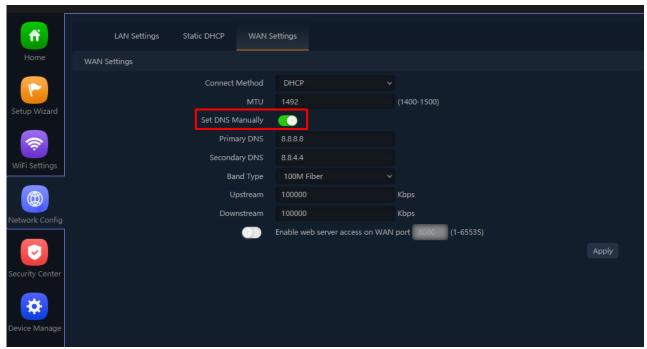
Fig 5.4.3 Set DNS manually for AirONE AIR-CPE1K+
