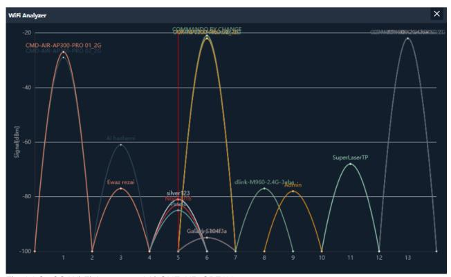
Fig 4.1.3 2G Wi-Fi Analyzer of AirONE AIR-CPE1K+
