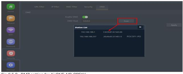
Fig 6.5.2 DMZ setting for AirONE AIR-CPE1K+
