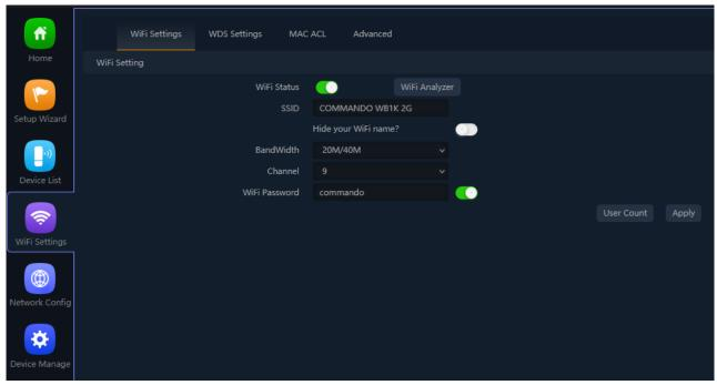
Fig 4.1.1 2G Basic Wi-Fi of AirONE AIR-CPE1K+
