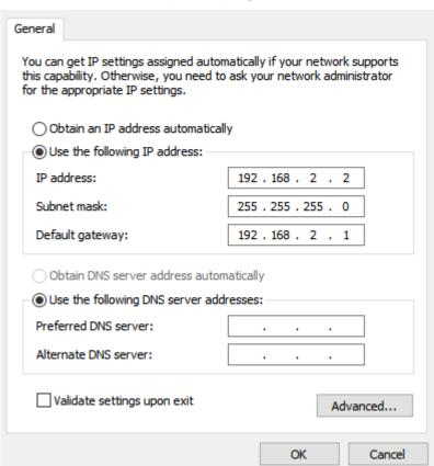
Fig 3. IP setting in PC to access AirONE AIR-CPE1K+ for New version
