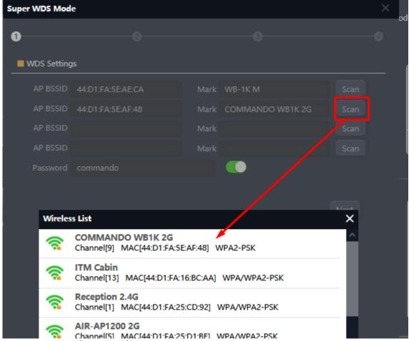
Fig 2.2.2 Scan (AP BSSID) Bridges/AP for connecting AirONE AIR-CPE1K+
