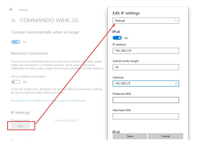
Fig 5. Edit IP setting from DHCP to Manual as shown for COMMANDO WB1K 2G SSID 14
