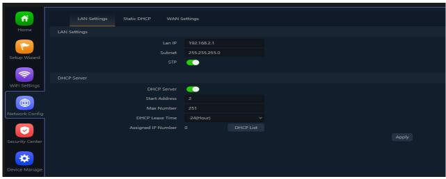
Fig 5.1.1 Setting LAN IP which used as access IP for AirONE AIR-CPE1K+
