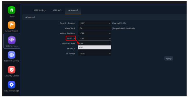
Fig 4.4.5 Setting Short GI for AirONE AIR-CPE1K+
