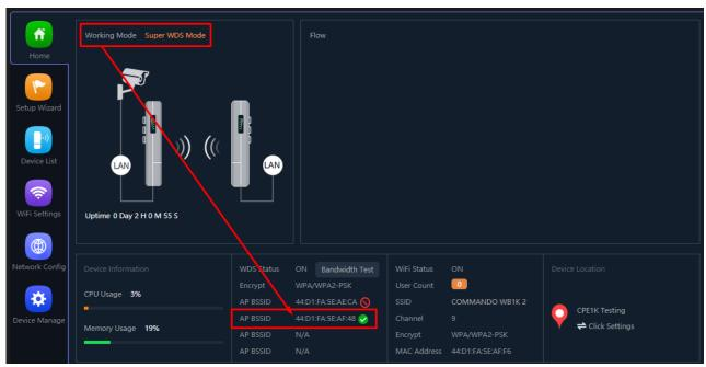
Fig 2.2.6 Active Super WDS mode of AirONE AIR-CPE1K+
