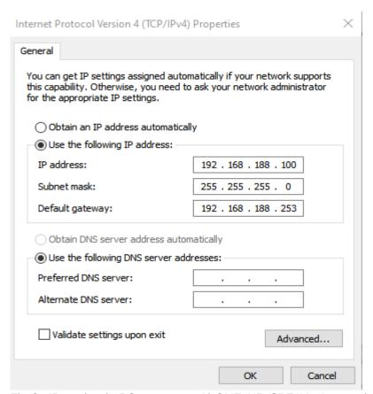
Fig 2. IP setting in PC to access AirONE AIR-CPE1K+ for previous version
