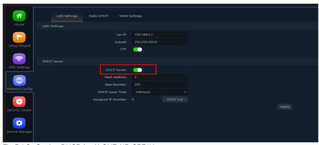
Fig 5.1.2 Setting DHCP for AirONE AIR-CPE1K+
