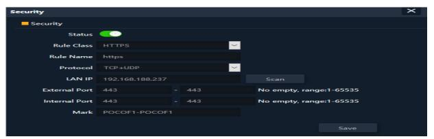
Fig 6.4.2 Security Rules setting for AirONE AIR-CPE1K+
