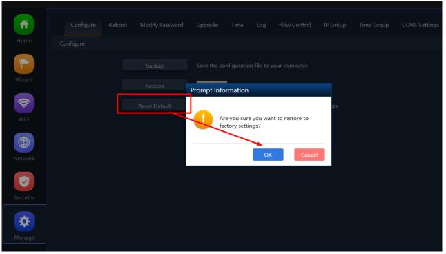
Fig 7.1.4 Reset to factory default for AirONE AIR-CPE1K+
