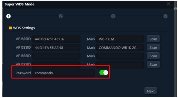
Fig 2.2.3 Super WDS mode scan Bridges/ SSID for AirONE AIR-CPE1K+
