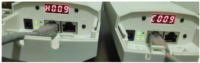
Fig 1. Physical port on AirONE AIR-CPE1K+
