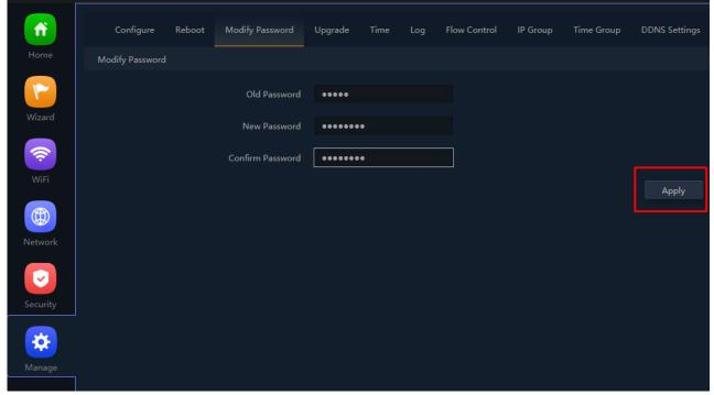
Fig 7.3.2 Setting New password for AirONE AIR-CPE1K+
