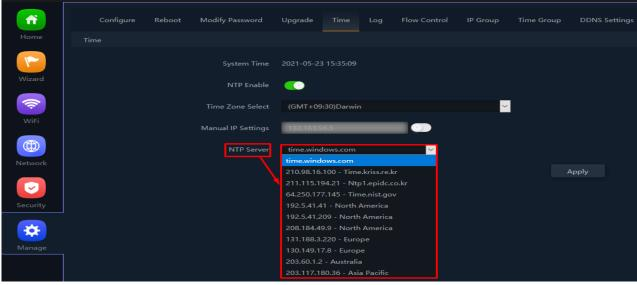
Fig 7.5.5 Selecting well know NTP server for AirONE AIR-CPE1K+
