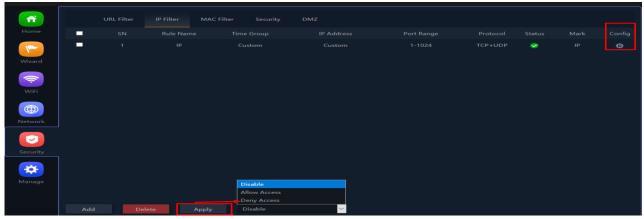
Fig 6.2.3 IP filter setting for AirONE AIR-CPE1K+
