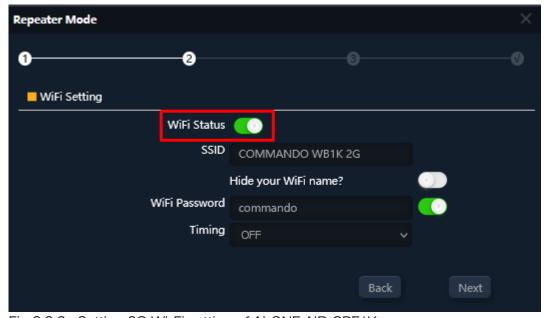
Fig 2.3.3 Setting 2G Wi-Fi setting of AirONE AIR-CPE1K+
