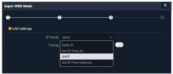
Fig 2.2.4 LAN Setting Super WDS mode of AirONE AIR-CPE1K+
