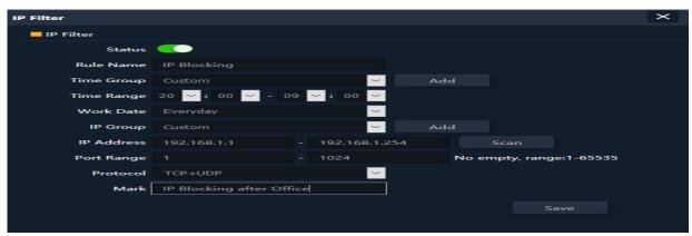
Fig 6.2.2 Setting IP filter for AirONE AIR-CPE1K+
