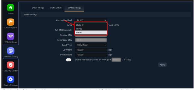
Fig 5.4.2 Changing Connect type manually for AirONE AIR-CPE1K+
