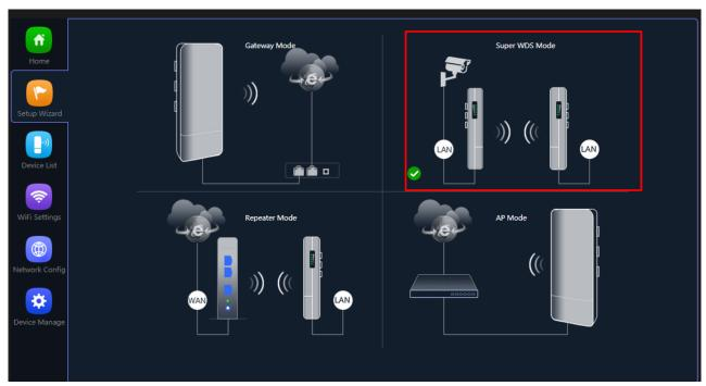
Fig 2.2.1 Super WDS mode of AirONE AIR-CPE1K+
