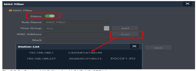
Fig 6.3.2 Setting MAC filter for AirONE AIR-CPE1K+
