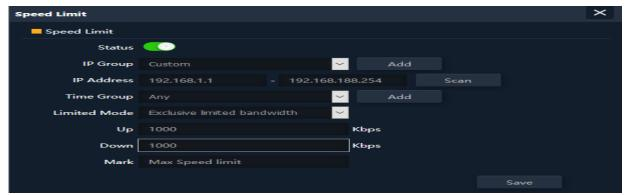
Fig 7.7.2 Enabling Speed limit for AirONE AIR-CPE1K+
