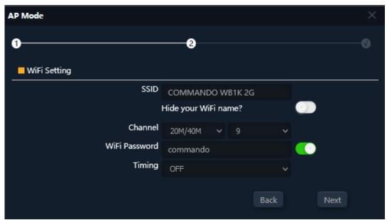
Fig 2.4.3 Setting 2G Wi-Fi for AP mode of AirONE AIR-CPE1K+
