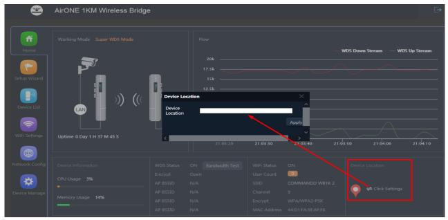
Fig 1.1.2 Changing Device Description of AirONE AIR-CPE1K+
