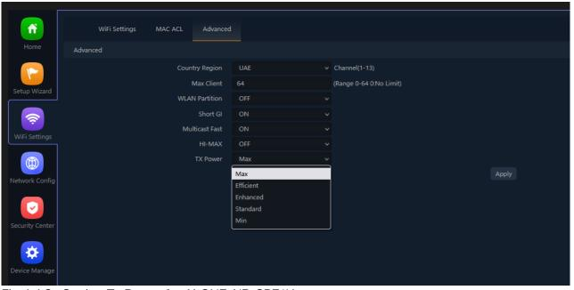
Fig 4.4.8 Setting Tx Power for AirONE AIR-CPE1K+
