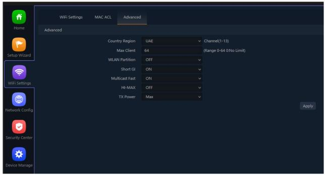
Fig 4.4.1 Default Advanced setting for AirONE AIR-CPE1K+
