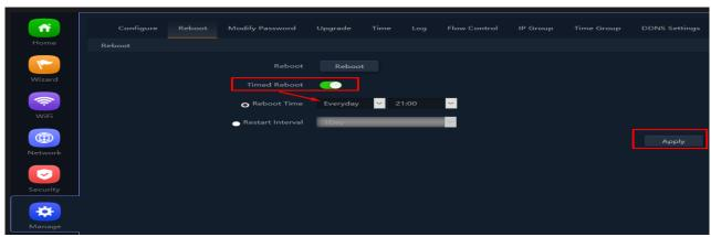
Fig 7.2.4 Enable daily reboot for AirONE AIR-CPE1K+
