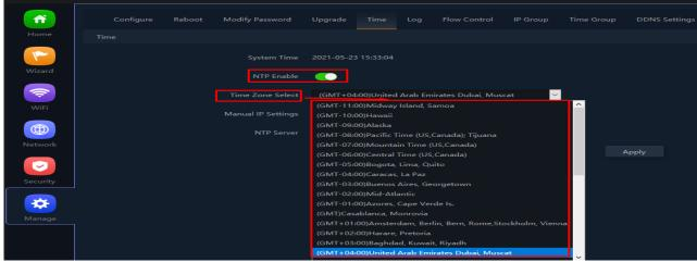
Fig 7.5.3 Enable NTP and select time zone for AirONE AIR-CPE1K+
