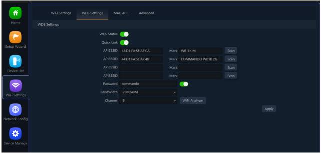
Fig 4.2.1 Scan 2G Repeater SSID AirONE AIR-CPE1K+
