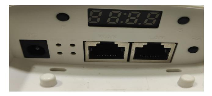
Fig 1. Physical port on AirONE AIR-CPE1K+
