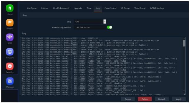
Fig 7.6.4 Enabling Remote Log server setting IP for AirONE AIR-CPE1K+
