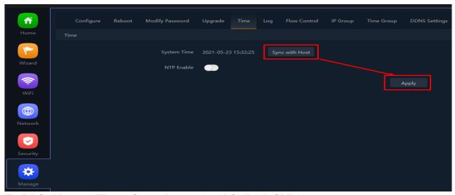
Fig 7.5.2 Disable NTP and Sync with host for AirONE AIR-CPE1K+
