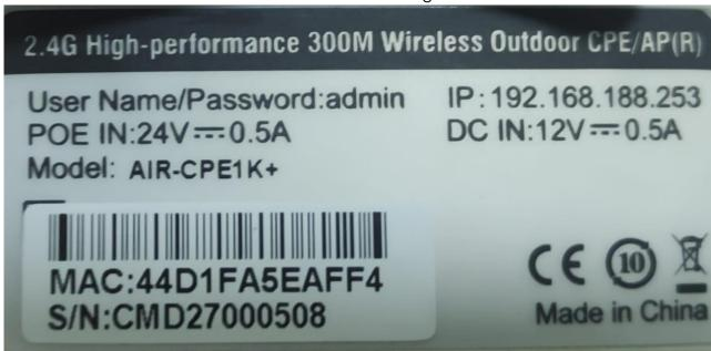
Fig 2. Access IP of AirONE AIR-CPE1K+
