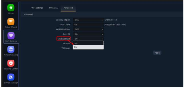
Fig 4.4.6 Setting Multicast Fast for AirONE AIR-CPE1K+
