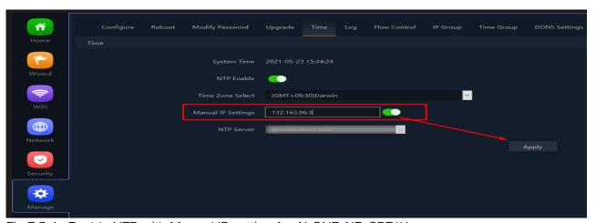
Fig 7.5.4 Enable NTP with Manual IP setting for AirONE AIR-CPE1K+
