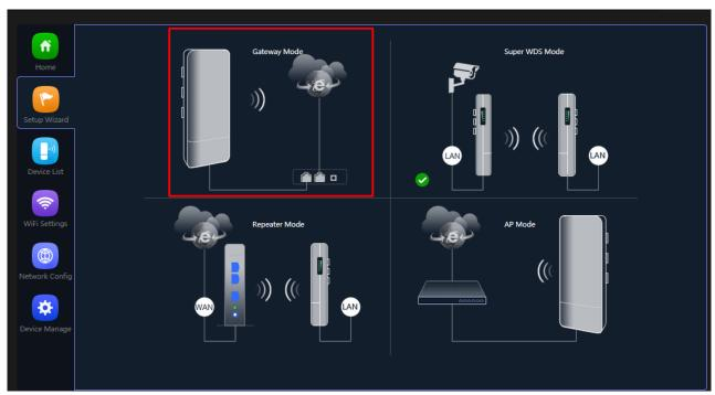
Fig 2.1.1 Gateway mode of AirONE AIR-CPE1K+
