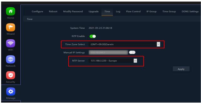
Fig 7.5.6 NTP server for AirONE AIR-CPE1K+
