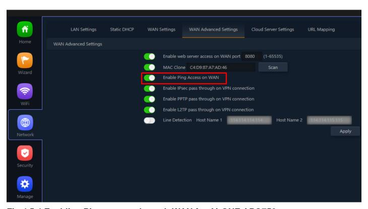
Fig 4.5.4 Enabling Ping access through WAN for AirONE APO750
