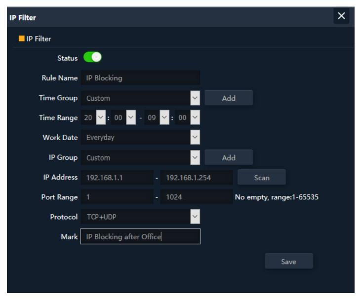
Fig 5.2.2 Setting IP filter for AirONE APO750
