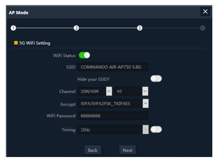
Fig 2.4.4 Setting 5G Wi-Fi for AP mode of AirONE APO750 (This image is for reference purpose only)
