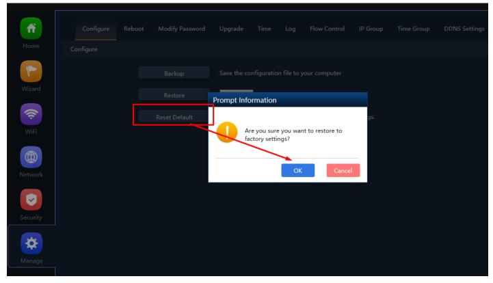
Fig 6.1.4 Reset to factory default for AirONE APO75
