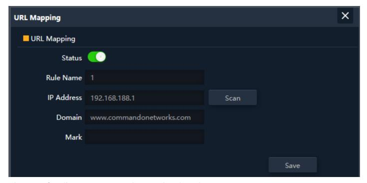
Fig 4.7.2 Configure URL Mapping setting for AirONE APO750
