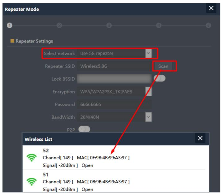
Fig 2.3.3 Selecting 5G Repeater SSID of AirONE APO750
