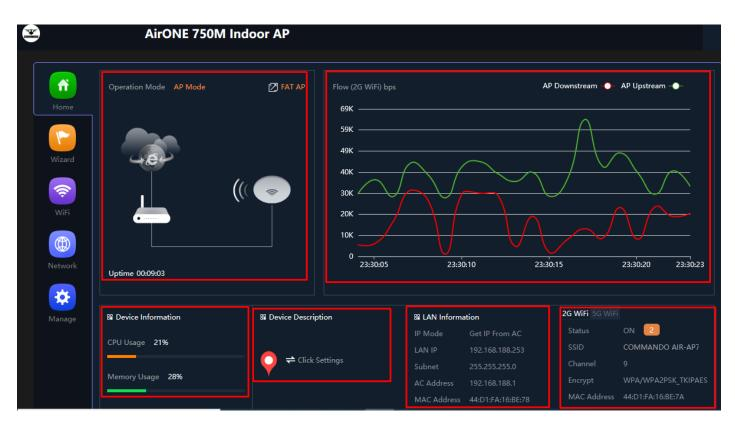
Fig 1.1 Home page Components of AirONE APO750 (This image is for reference purpose only)
