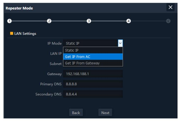
Fig 2.3.5 Setting LAN setting in repeater mode of AirONE APO750
