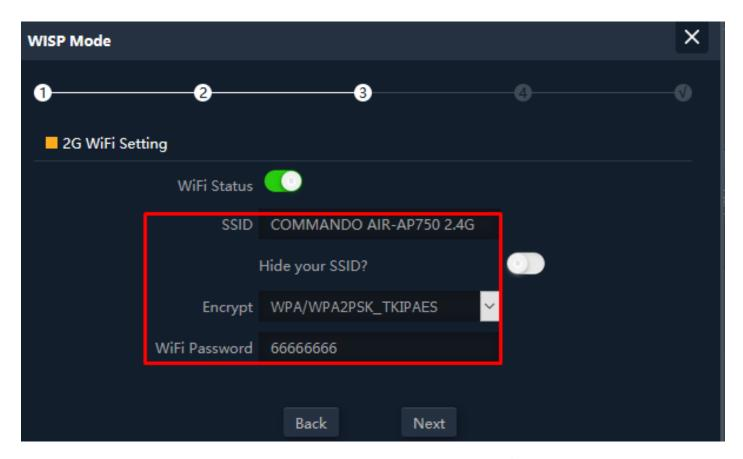
Fig 2.3.6 2G Wi-Fi Setting WISP mode of AirONE APO750 (This image is for reference purpose only)
