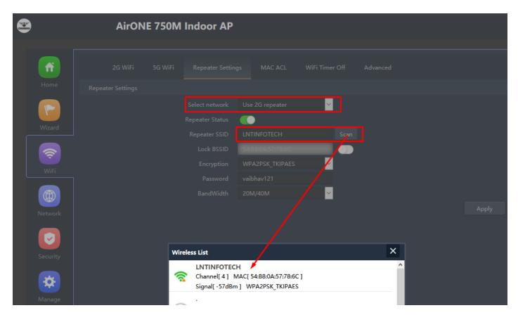
Fig 3.2.1 Scan 2G Repeater SSID AirONE APO750 (This image is for reference purpose only)
