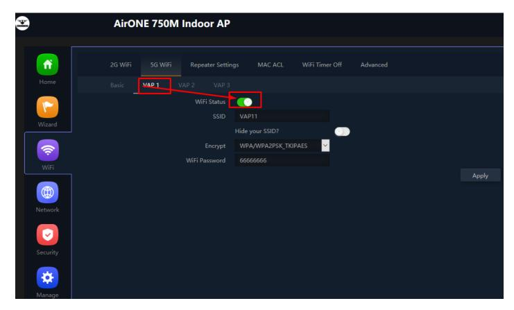
Fig 3.1.8 Enabling 5G VAP 1 of AirONE APO750 (This image is for reference purpose only)
