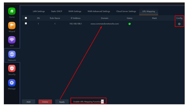
Fig 4.7.3 URL Mapping setting for AirONE APO750
