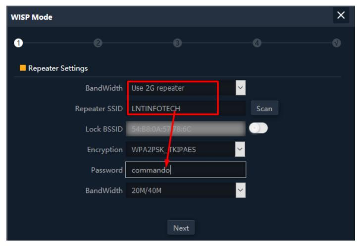
Fig 2.3.4 Repeater SSID for 2G repeater WISP mode of AirONE APO750
