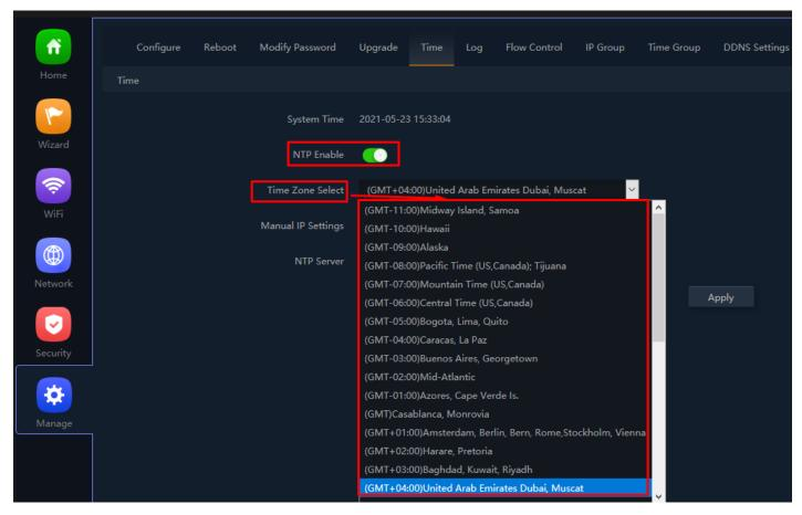
Fig 6.5.3 Enable NTP and select time zone for AirONE APO750
