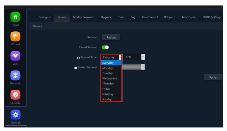
Fig 6.2.3 Enable timed reboot for AirONE APO750
