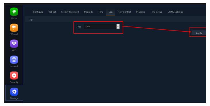
Fig 6.6.2 Turning OFF Log setting for AirONE APO750
