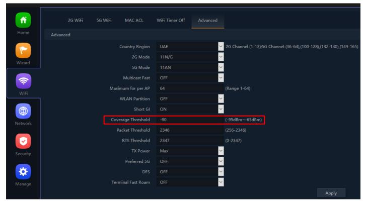
Fig 3.5.9 Setting Coverage Threshold for AirONE APO750
