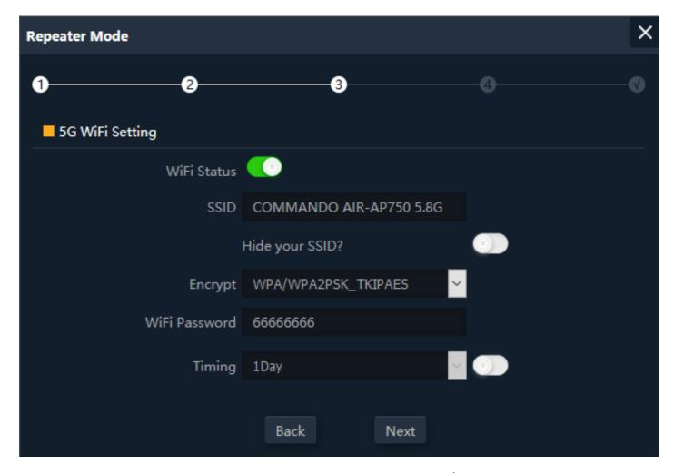
Fig 2.3.5 Setting 5G Wi-Fi setting of AirONE APO750 (This image is for reference purpose only)
