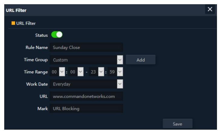
Fig 5.1.2 Setting URL filter for AirONE APO750
