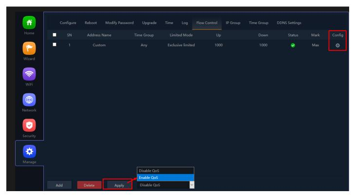
Fig 6.7.3 Flow control page for AirONE APO750
