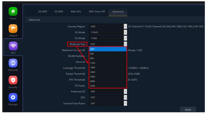
Fig 3.5.5 Selecting Multicast Fast for AirONE APO750
