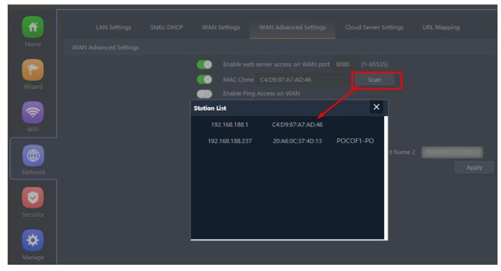
Fig 4.5.3 Configuration of MAC clone for AirONE APO750
