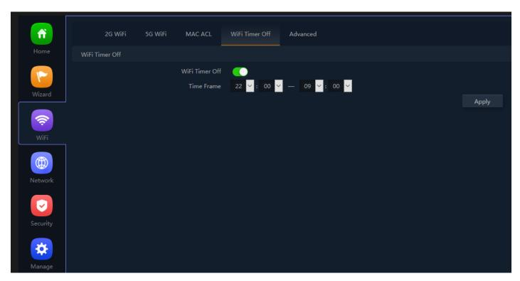
Fig 3.4.2 Wi-Fi Timer Off for AirONE APO750
