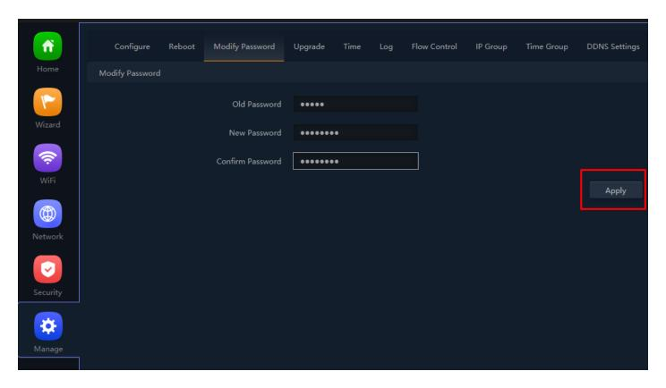
Fig 6.3.2 Setting New password for AirONE APO750
