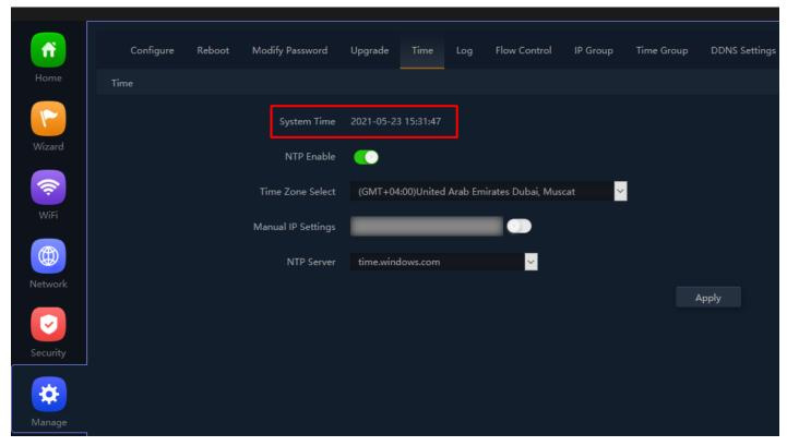
Fig 6.5.1 System Time for AirONE APO750
