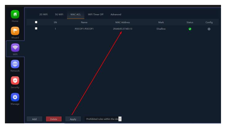
Fig 3.3.4 Apply MAC ACL for AirONE APO750
