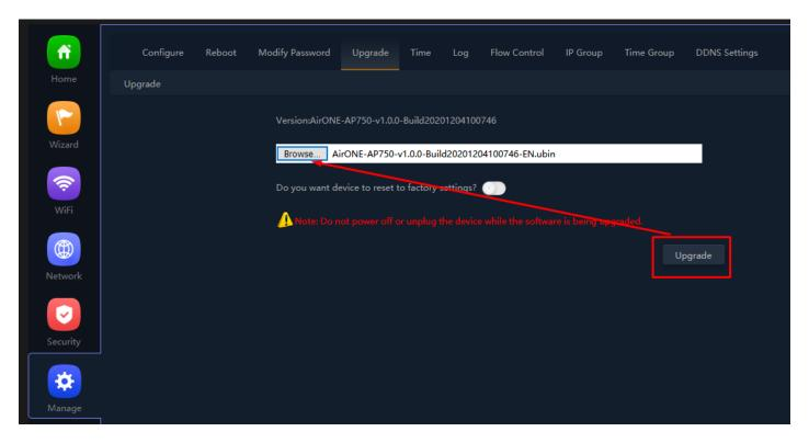
Fig 6.4.2 Browse for Upgrade file of connected PC for AirONE APO750 (This image is for reference purpose only)
