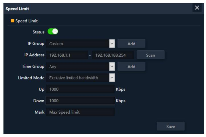
Fig 6.7.2 Enabling Speed limit for AirONE APO750
