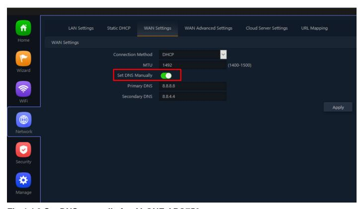
Fig 4.4.3 Set DNS manually for AirONE APO750
