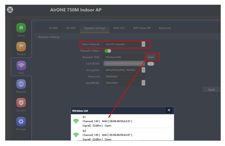
Fig 3.2.2 Scan 5G Repeater SSID AirONE APO750 (This image is for reference purpose only)
