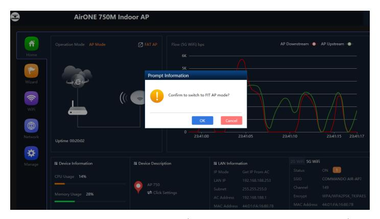
Fig 1.5.1 Fat AP mode of AirONE APO750 (This image is for reference purpose only)
