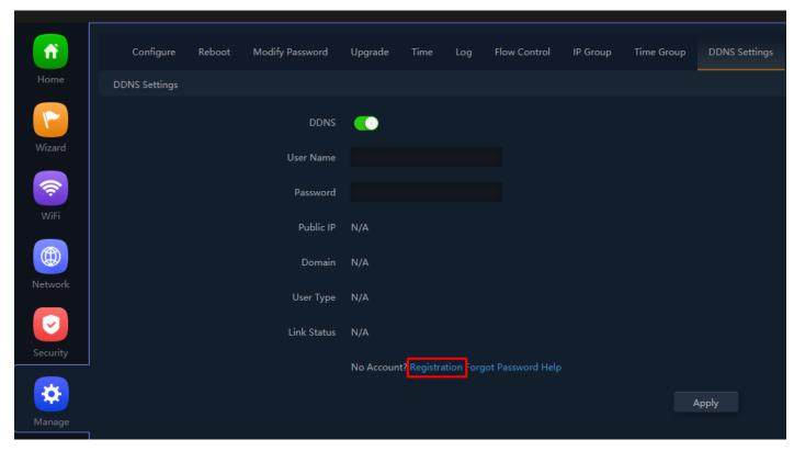
Fig 6.10.2 Enable DDNS page for AirONE APO750
