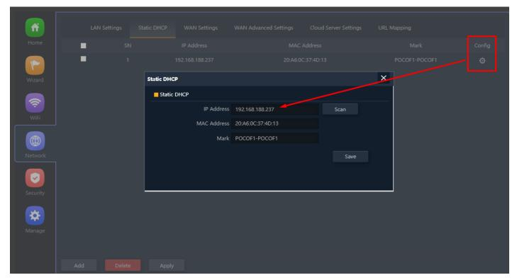
Fig 4.3.5 Config Button for Static DHCP for AirONE APO750
