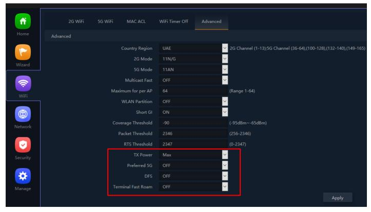
Fig 3.5.11 Setting Preferred 5G, DFS, Terminal Fast Roam for AirONE APO750
