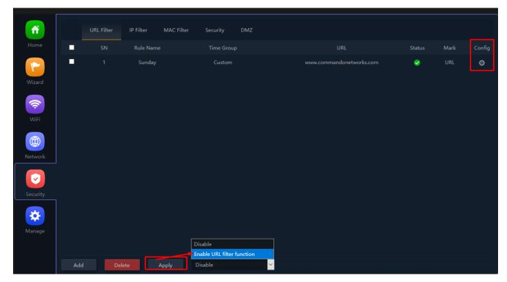
Fig 5.1.3 URL filter setting for AirONE APO750
