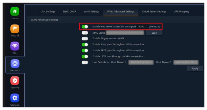
Fig 4.5.2 Enable Port setting for WEB server for AirONE APO750
