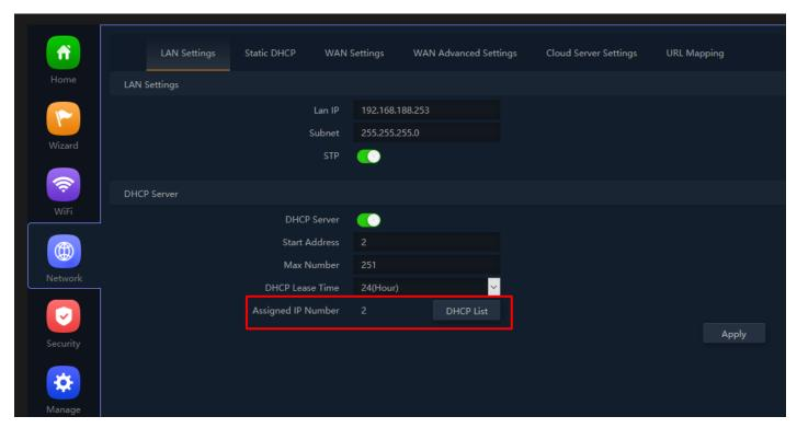
Fig 4.1.4 DHCP Assigned list for AirONE APO750
