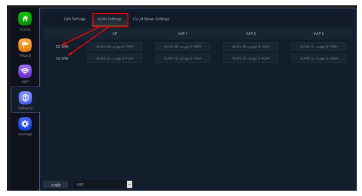
Fig 4.2.1 Default VLAN setting for AirONE APO750
