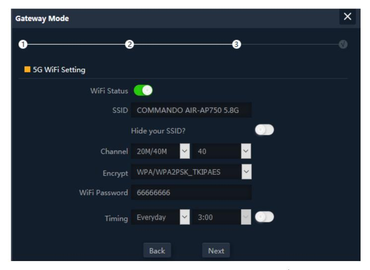
Fig 2.1.4 Gateway mode 5G Wi-Fi Setting of AirONE APO750 (This image is for reference purpose only)
