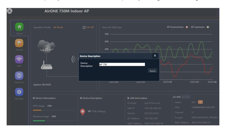
Fig 1.1.3 Changing Device Description of AirONE APO750 (This image is for reference purpose only)
