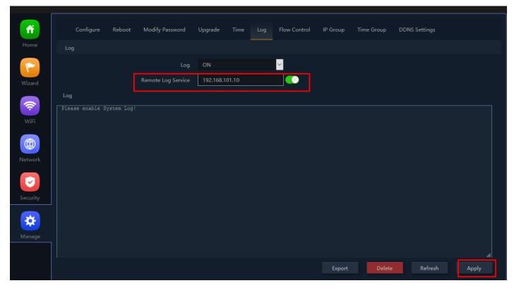
Fig 6.6.3 Remote Log service setting IP for AirONE APO750
