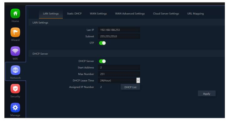
Fig 4.1.1 Setting LAN IP which used as access IP for AirONE APO750
