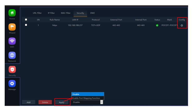
Fig 5.4.3 Security setting for AirONE APO750
