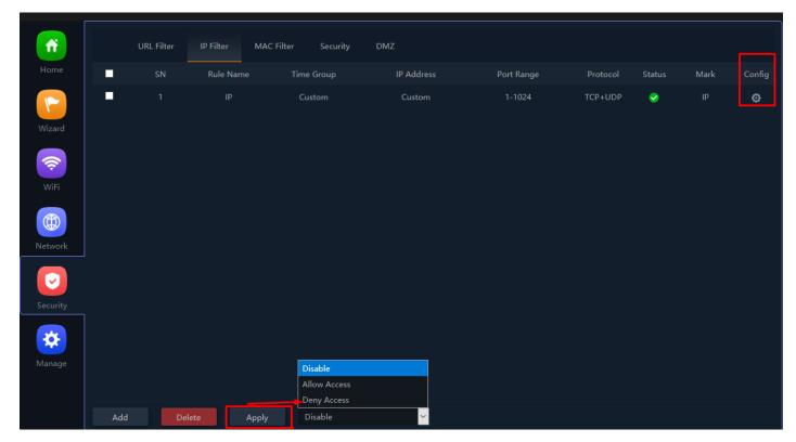
Fig 5.2.3 IP filter setting for AirONE APO750
