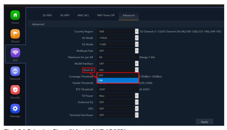
Fig 3.5.8 Selecting Short GI for AirONE APO750
