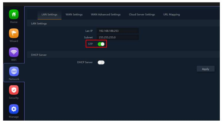
Fig 4.1.2 Enabling STP for AirONE APO750
