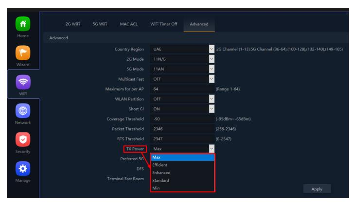
Fig 3.5.10 Setting Tx Power for AirONE APO750
