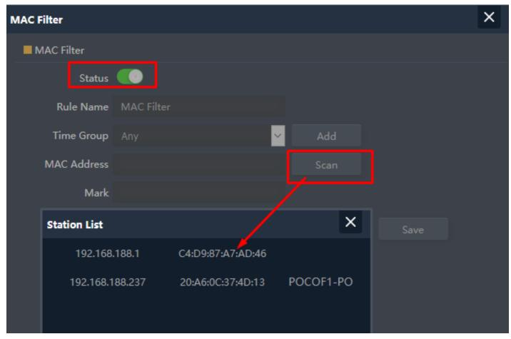
Fig 5.3.2 Setting MAC filter for AirONE APO750
