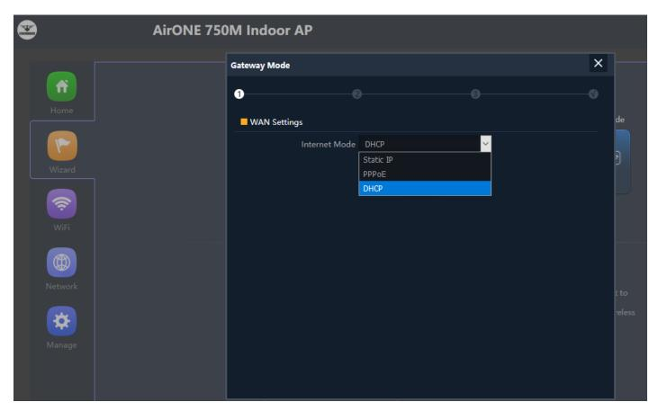
Fig 2.1.2 Gateway mode WAN Setting of AirONE APO750
