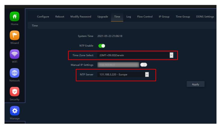
Fig 6.5.6 NTP server for AirONE APO750
