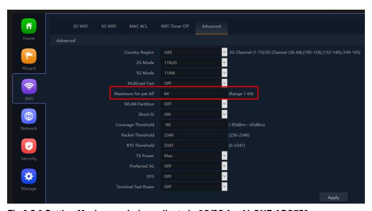
Fig 3.5.6 Setting Maximum wireless clients in 2G/5G for AirONE APO750
