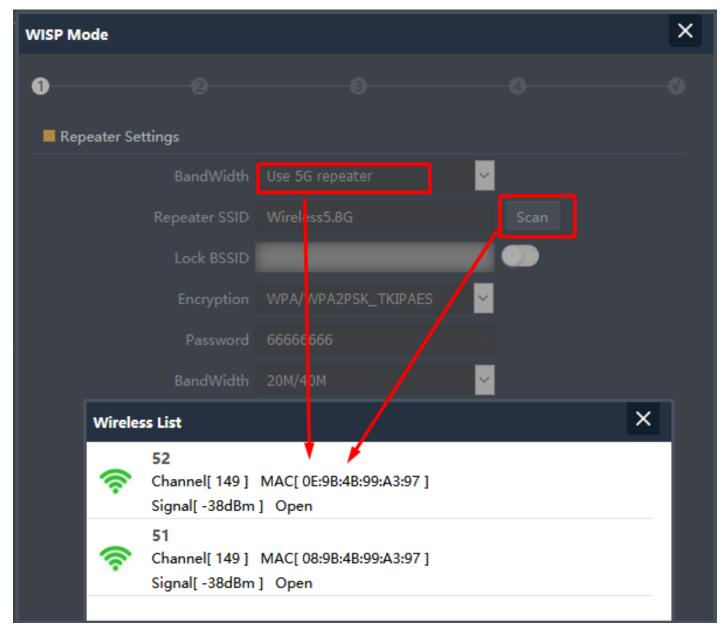
Fig 2.3.3 5G Repeater Setting WISP mode of AirONE APO750
