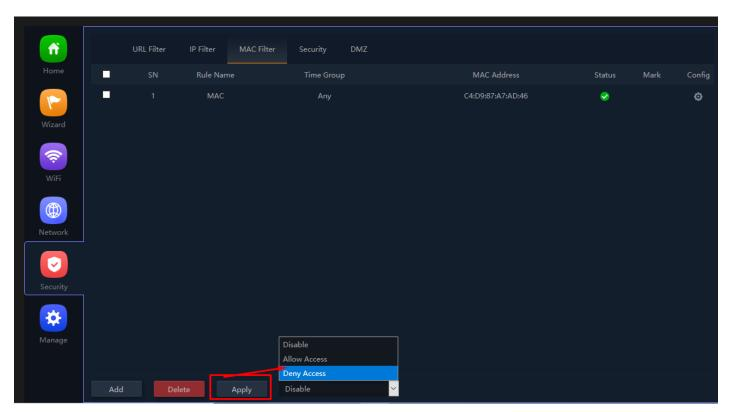
Fig 5.3.3 MAC filter setting for AirONE APO750
