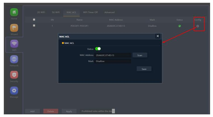
Fig 3.3.5 Config Button of MAC ACL for AirONE APO750
