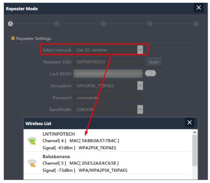
Fig 2.3.2 Selecting 2G Repeater SSID of AirONE APO750
