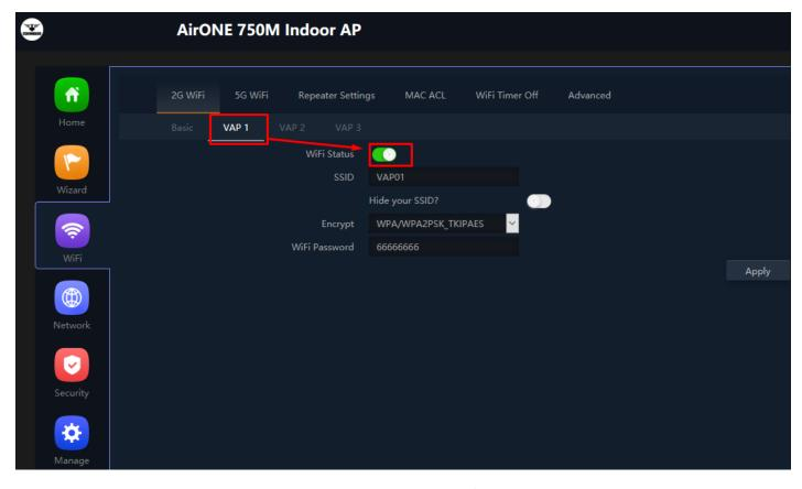
Fig 3.1.7 Enabling 2G VAP 1 of AirONE APO750 (This image is for reference purpose
