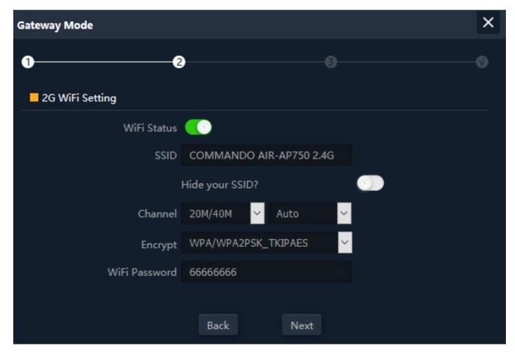
Fig 2.1.3 Gateway mode 2G Wi-Fi Setting of AirONE APO750 (This image is for reference purpose only)
