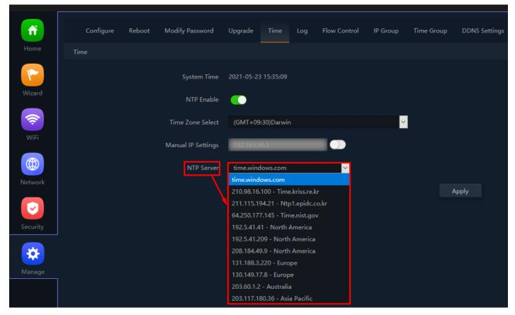
Fig 6.5.5 Selecting well know NTP server for AirONE APO750
