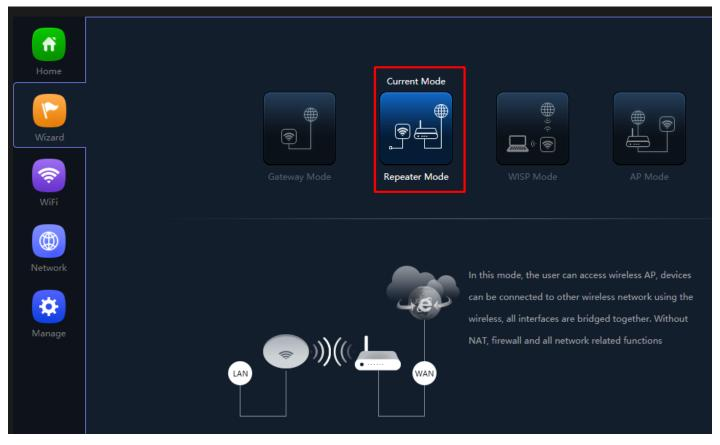
Fig 2.3.1 Repeater mode of AirONE APO750
