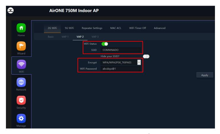
Fig 3.1.9 Enabling 2G Wi-Fi VAP 2 of AirONE APO750 (This image is for reference purpose only)
