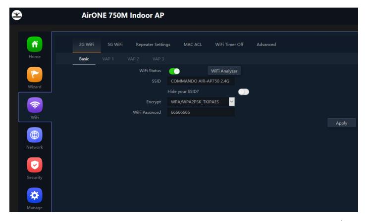
Fig 3.1.1 2G Wi-Fi enable and disable of Basic and VAP 1,2,3 of AirONE APO750 (This image is for reference purpose only)
