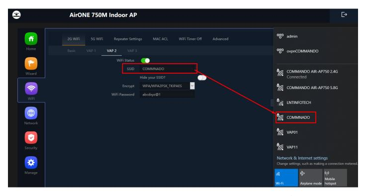
Fig 3.1.10 Wireless VAP 2 named COMMANDO of AirONE APO750 (This image is for reference purpose only)
