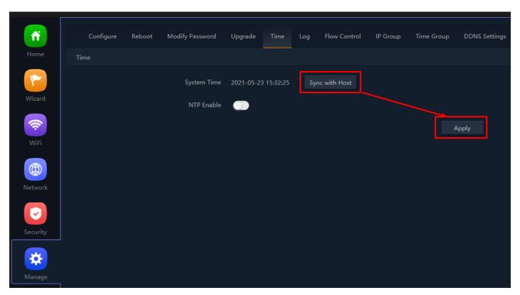
Fig 6.5.2 Disable NTP and Sync with host for AirONE APO750
