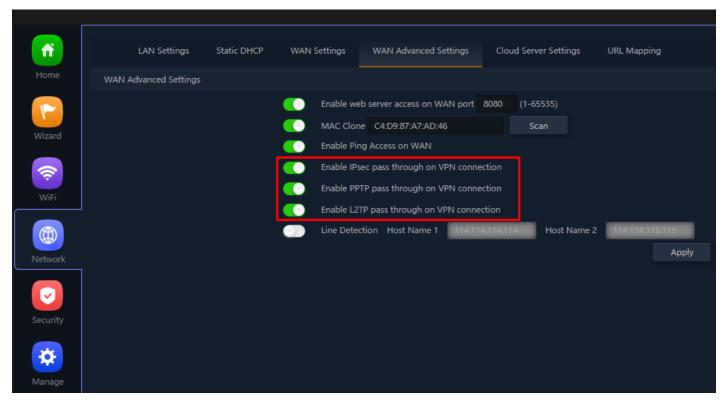
Fig 4.5.5 Enabling IPSec/PPTP/L2TP access through VPN for AirONE APO750
