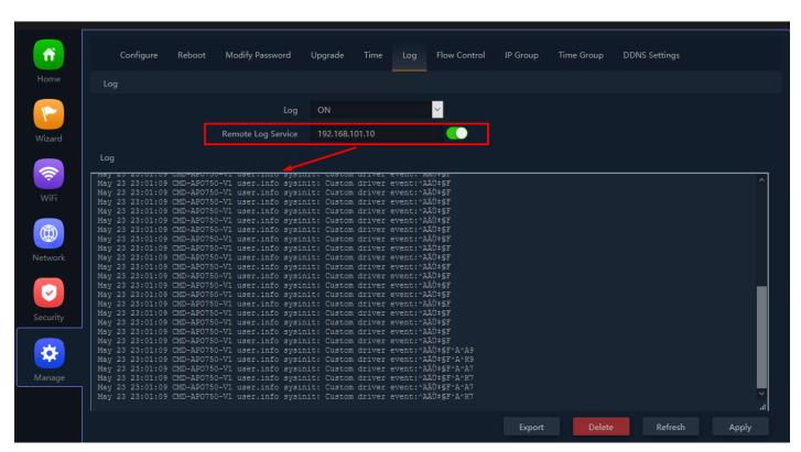
Fig 6.6.4 Enabling Remote Log server setting IP for AirONE APO750
