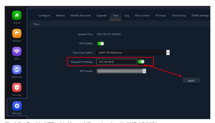
Fig 6.5.4 Enable NTP with Manual IP setting for AirONE APO750
