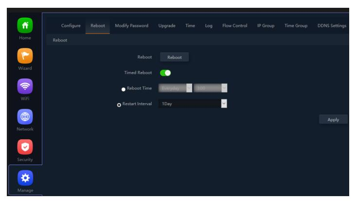
Fig 6.2.5 Enable Restart interval for AirONE APO750
