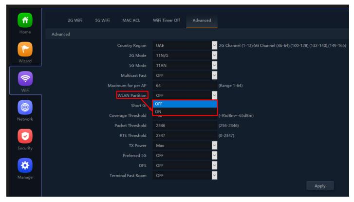
Fig 3.5.7 Selecting WLAN Partition for AirONE APO750
