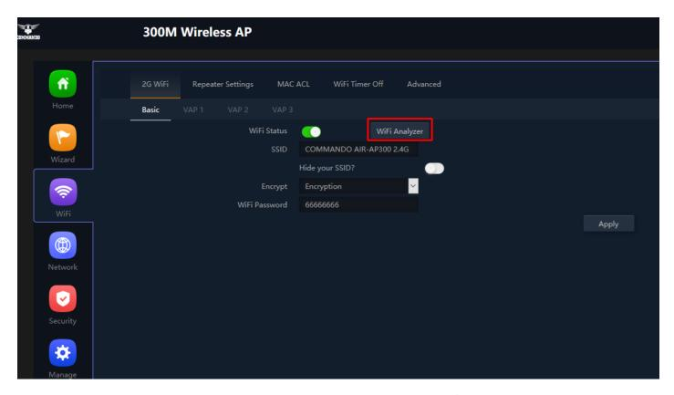
Fig 3.1.3 2G Wi-Fi Analyzer button of AirONE APO750 (This image is for reference purpose only)
