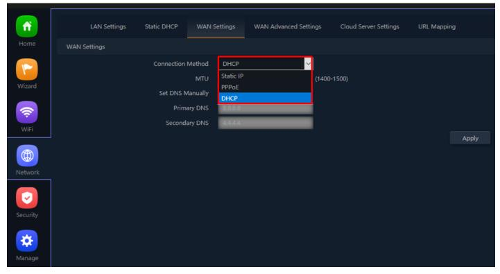
Fig 4.4.2 Changing Connect type manually for AirONE APO750
