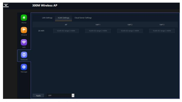
Fig 4.2.1 Default VLAN setting for AirONE APO300
