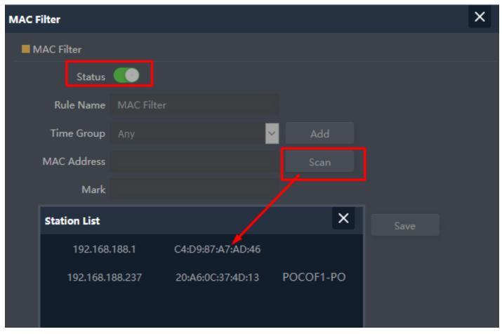
Fig 5.3.2 Setting MAC filter for AirONE APO300
