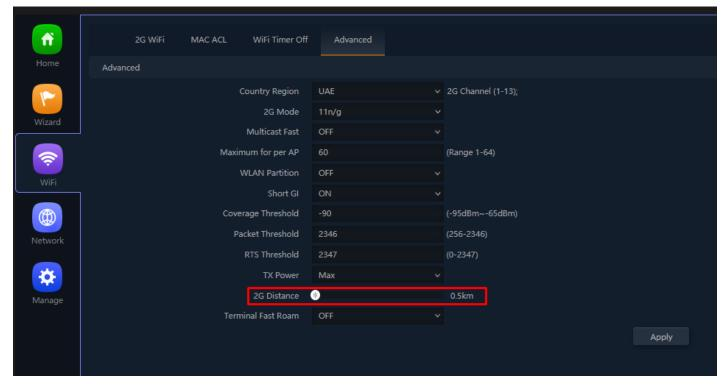
Fig 3.5.11 Setting 2G distance for AirONE APO300
