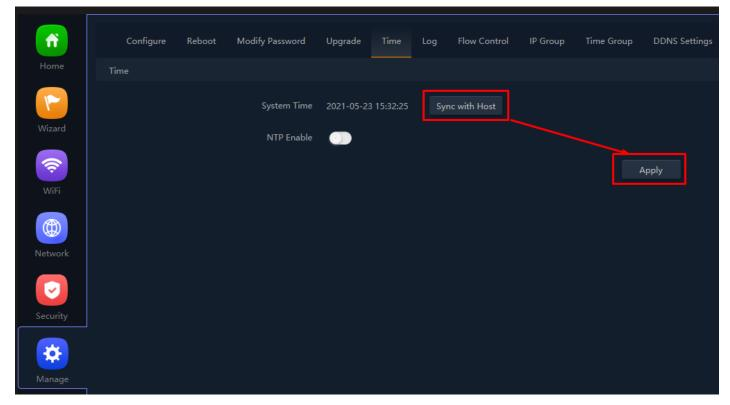
Fig 6.5.2 Disable NTP and Sync with host for AirONE APO300
