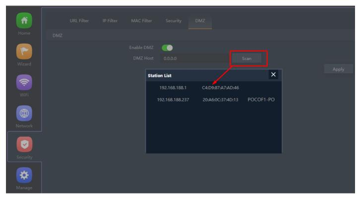
Fig 5.5.2 DMZ setting for AirONE APO300
