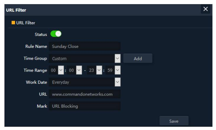
Fig 5.1.2 Setting URL filter for AirONE APO300
