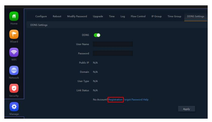
Fig 6.10.2 Enable DDNS page for AirONE APO300
