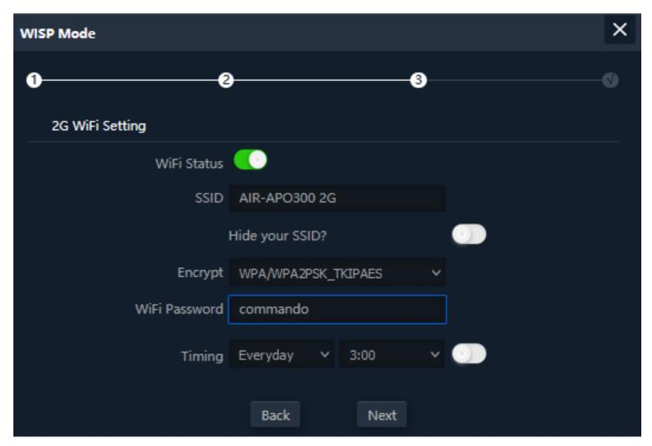
Fig 2.3.4 2G Wi-Fi Setting WISP mode of AirONE APO300
