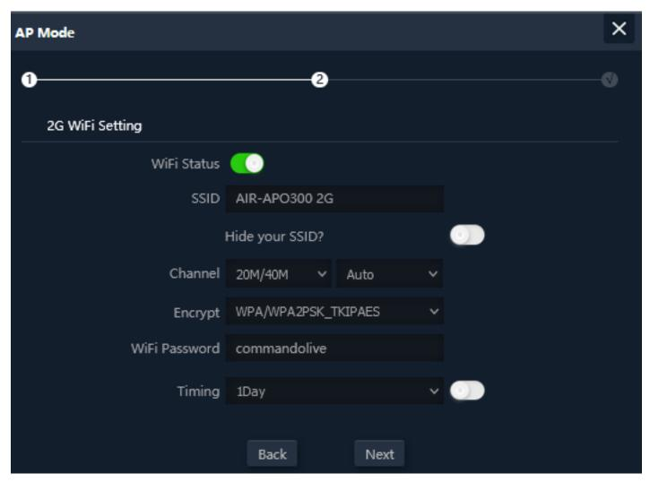
Fig 2.5.3 Setting 2G Wi-Fi for AP mode of AirONE APO300
