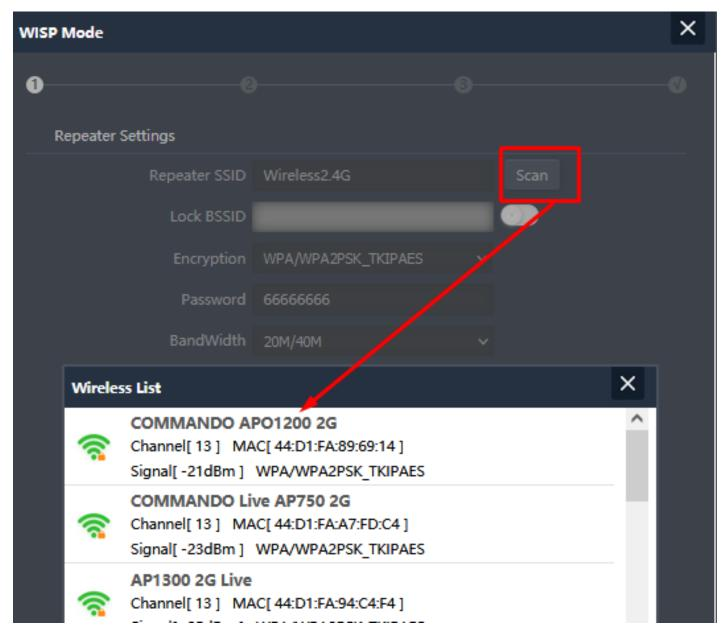
Fig 2.3.2 Repeater Setting WISP mode of AirONE APO300
