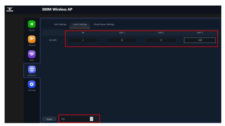
Fig 4.2.2 VLAN setting for AirONE APO300
