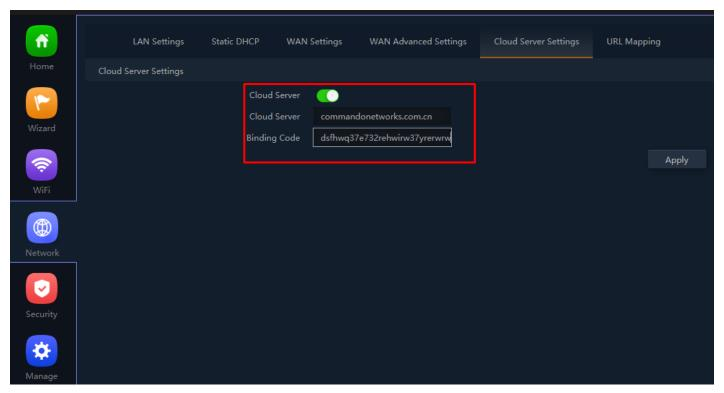
Fig 4.6.2 Enabling Cloud server setting for AirONE APO30
