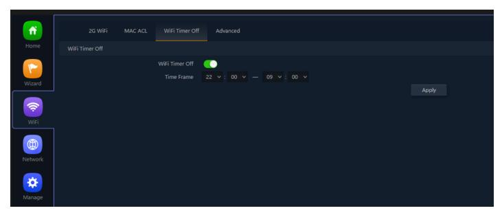
Fig 3.4.2 Wi-Fi Timer Off for AirONE APO300
