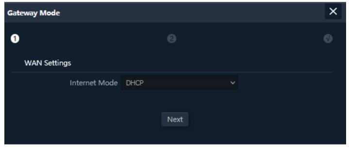
Fig 2.1.2 Gateway mode WAN Setting of AirONE APO300
