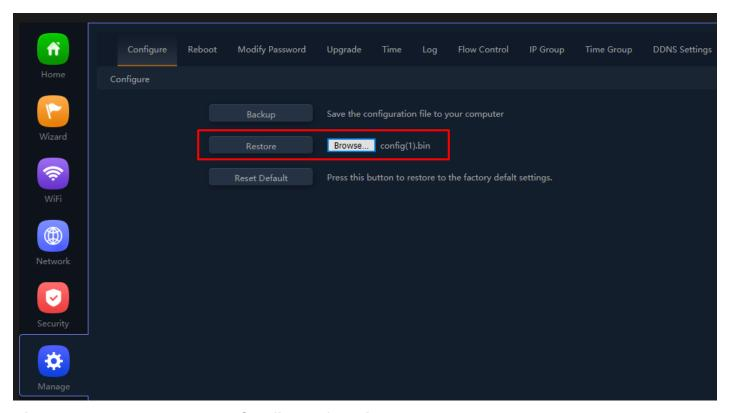
Fig 6.1.3 Restore to known Configure for AirONE APO300
