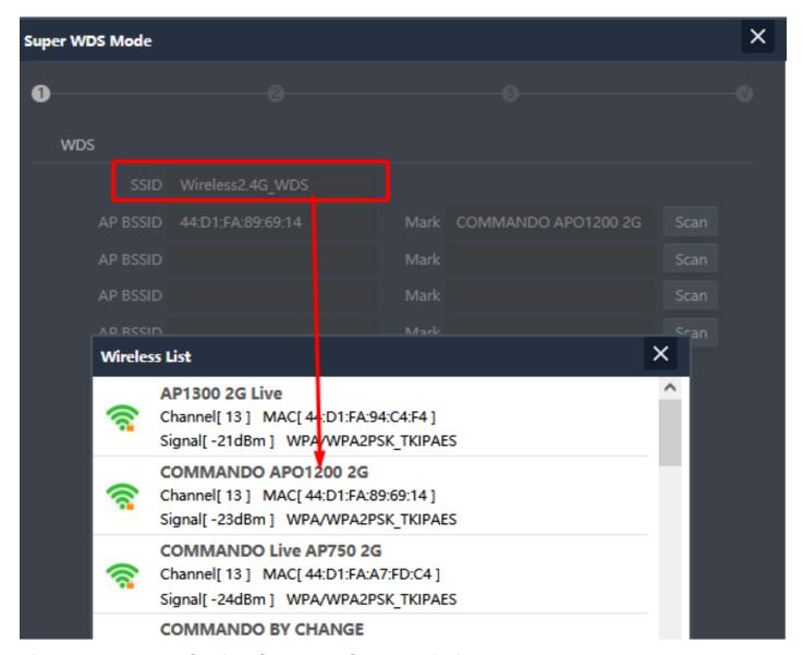
Fig 2.2.2 Repeater Setting Super WDS Mode of AirONE APO300
