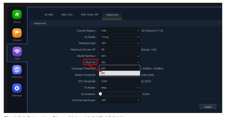
Fig 3.5.8 Selecting Short GI for AirONE APO300
