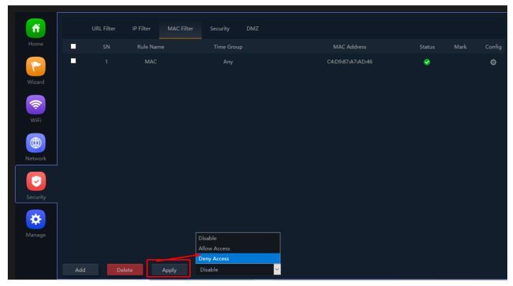
Fig 5.3.3 MAC filter setting for AirONE APO300
