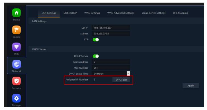
Fig 4.1.4 DHCP Assigned list for AirONE APO300
