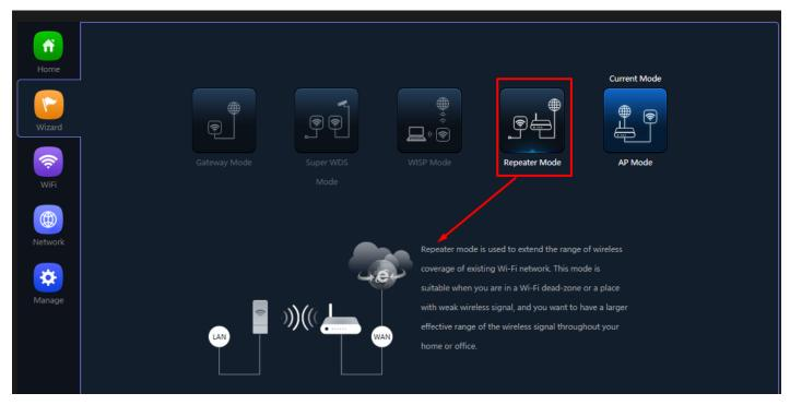
Fig 2.4.1 Repeater mode of AirONE APO300
