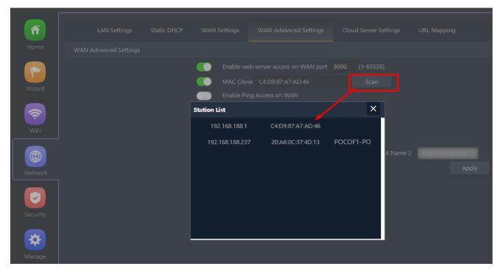
Fig 4.5.3 Configuration of MAC clone for AirONE APO300
