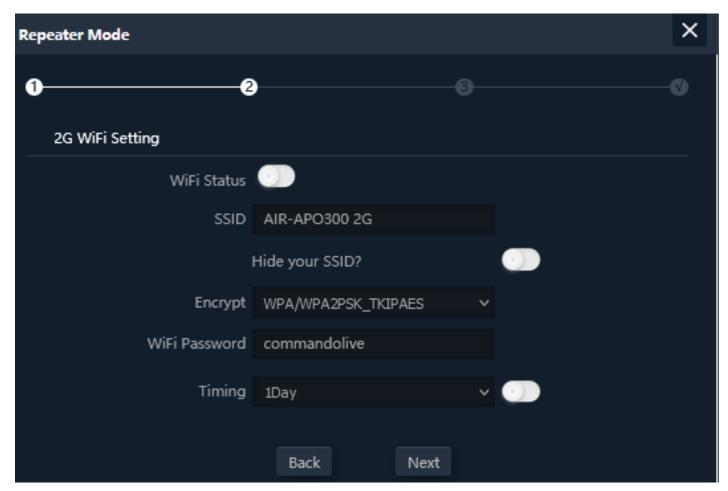
Fig 2.2.3 Setting 2G Wi-Fi setting of AirONE APO300
