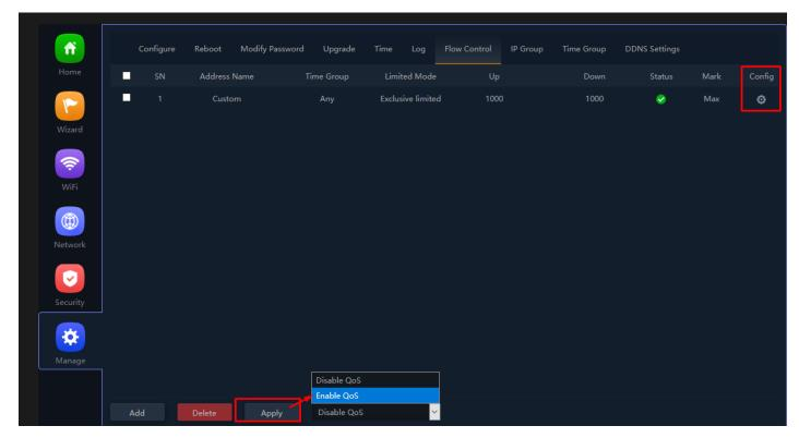
Fig 6.7.3 Flow control page for AirONE APO300
