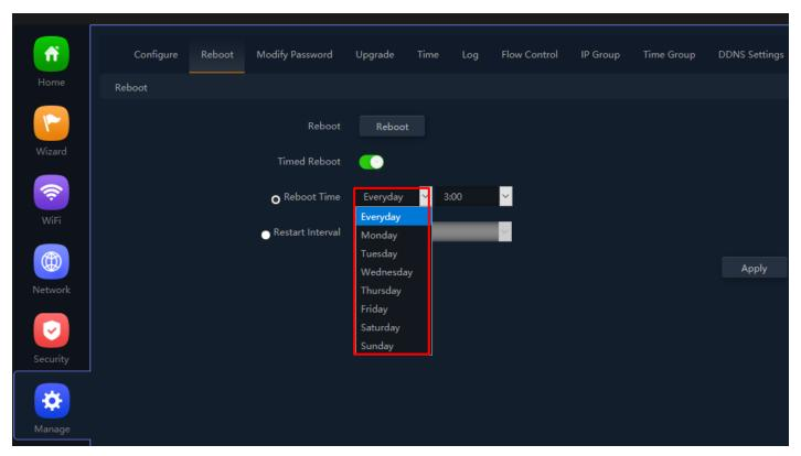
Fig 6.2.3 Enable timed reboot for AirONE APO300
