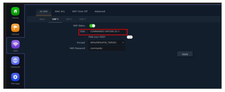
Fig 3.1.4 Enabling 2G VAP 1 of AirONE APO300
