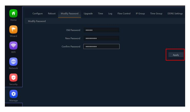
Fig 6.3.2 Setting New password for AirONE APO300
