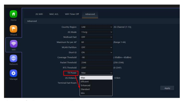
Fig 3.5.10 Setting Tx Power for AirONE APO300
