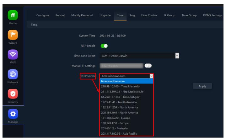
Fig 6.5.5 Selecting well know NTP server for AirONE APO300
