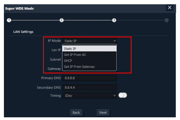
Fig 2.2.4 2G Wi-Fi Setting Super WDS mode of AirONE APO300
