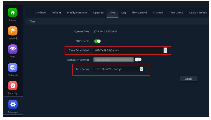
Fig 6.5.6 NTP server for AirONE APO300
