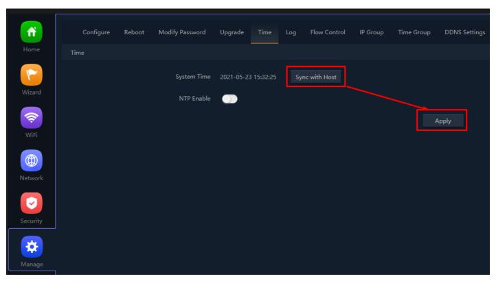
Fig 6.5.2 Disable NTP and Sync with host for AirONE AP750
