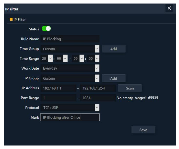
Fig 5.2.2 Setting IP filter for AirONE AP750
