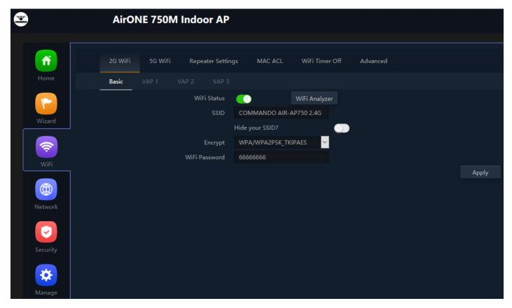
Fig 3.1.1 2G Wi-Fi enable and disable of Basic and VAP 1,2,3 of AirONE AP750
