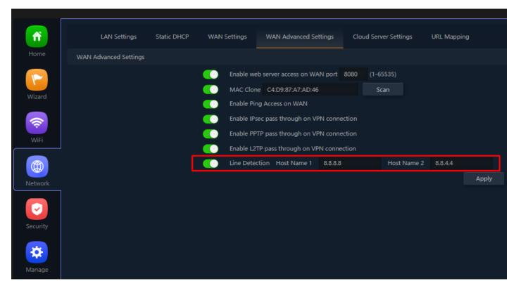
Fig 4.5.6 Line Detection for AirONE AP750
