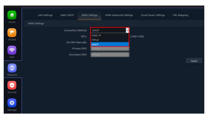
Fig 4.4.2 Changing Connect type manually for AirONE AP750
