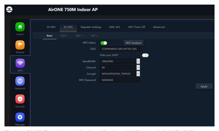
Fig 3.1.2 5G Wi-Fi enable and disable of Basic and VAP 1,2,3 of AirONE AP750
