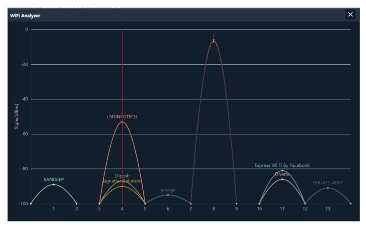
Fig 3.1.5 2G Wi-Fi Analyzer of AirONE AP750
