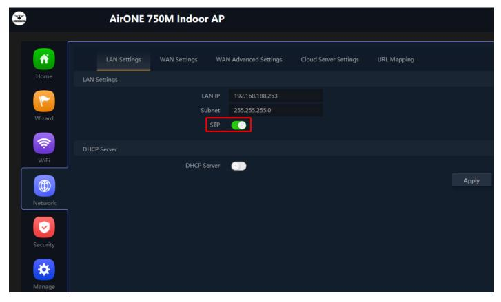
Fig 4.1.2 Enabling STP for AirONE AP750
