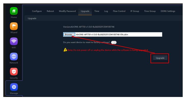
Fig 6.4.2 Browse for Upgrade file of connected PC for AirONE AP750
