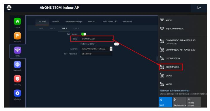
Fig 3.1.11 Wireless VAP 2 named COMMANDO of AirONE AP750
