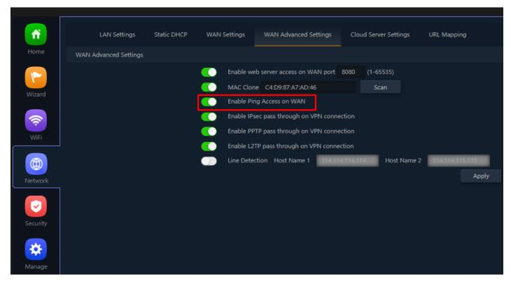
Fig 4.5.4 Enabling Ping access through WAN for AirONE AP750
