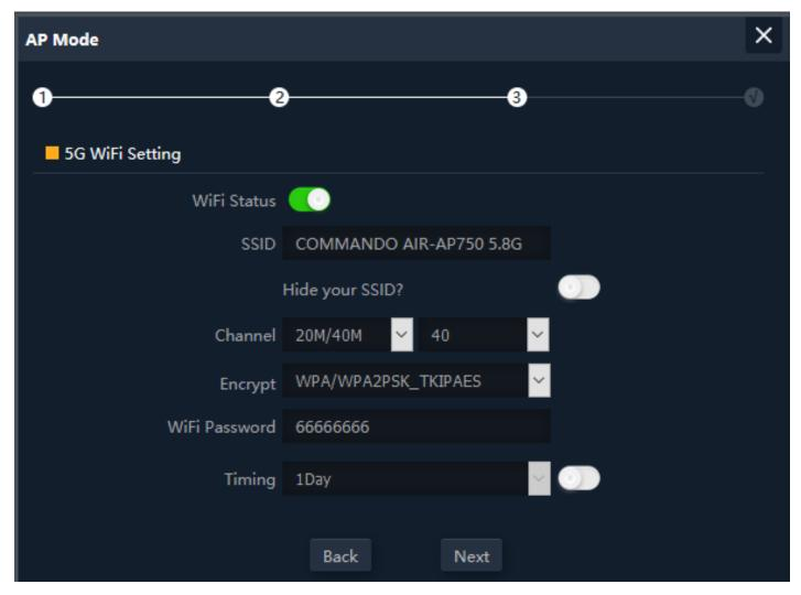
Fig 2.4.4 Setting 5G Wi-Fi for AP mode of AirONE AP750
