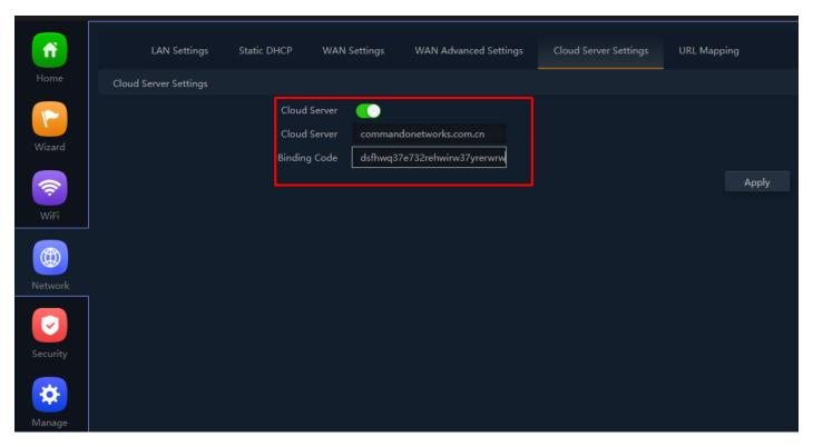
Fig 4.6.2 Enabling Cloud server setting for AirONE AP750
