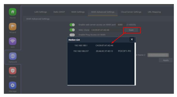
Fig 4.5.3 Configuration of MAC clone for AirONE AP750
