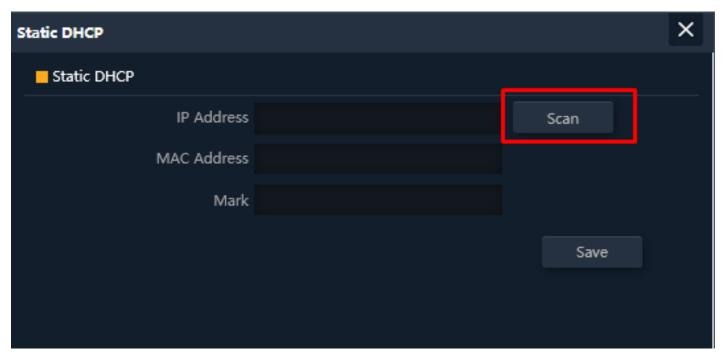
Fig 4.3.2 Static DHCP scan for AirONE AP750
