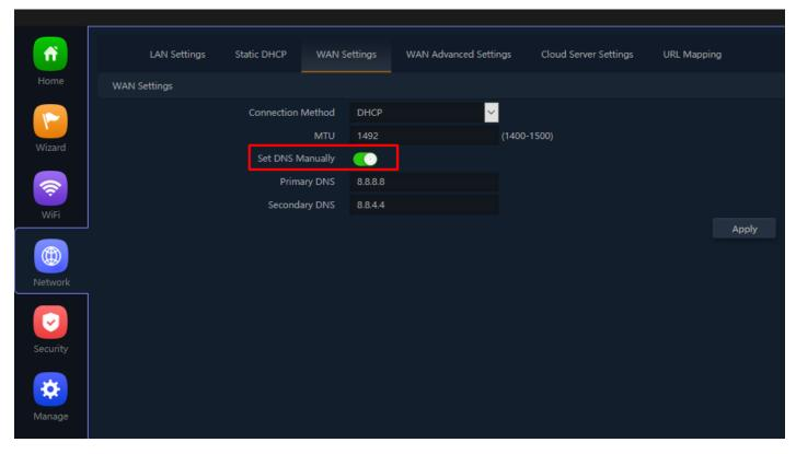
Fig 4.4.3 Set DNS manually for AirONE AP750
