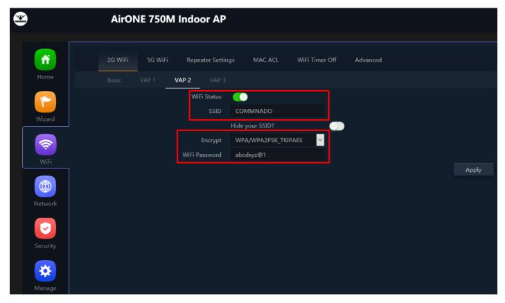
Fig 3.1.10 Enabling 2G Wi-Fi VAP 2 of AirONE AP750
