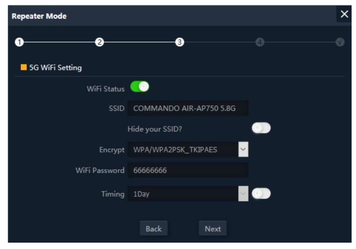
Fig 2.3.5 Setting 5G Wi-Fi setting of AirONE AP750
