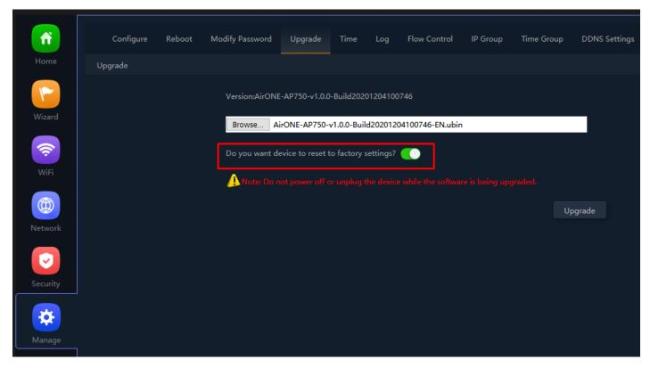
Fig 6.4.3 Upgrade with no previous configuration for AirONE AP750
