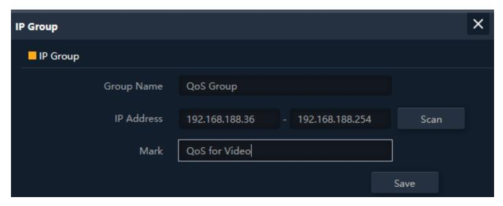
Fig 6.8.2 IP group name and associated IP address for AirONE AP750
