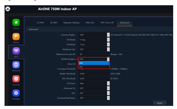
Fig 3.5.7 Selecting WLAN Partition for AirONE AP750
