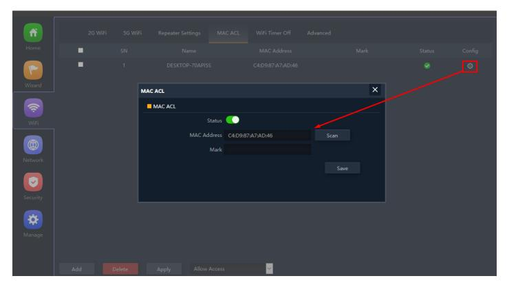
Fig 3.3.5 Config Button of MAC ACL for AirONE AP750
