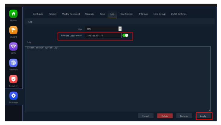
Fig 6.6.3 Remote Log service setting IP for AirONE AP750
