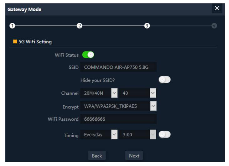
Fig 2.1.4 Gateway mode 5G Wi-Fi Setting of AirONE AP750
