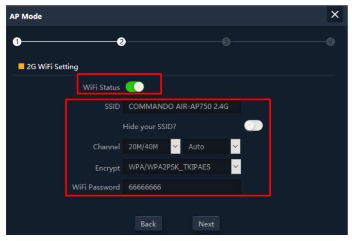
Fig 2.4.3 Setting 2G Wi-Fi for AP mode of AirONE AP750
