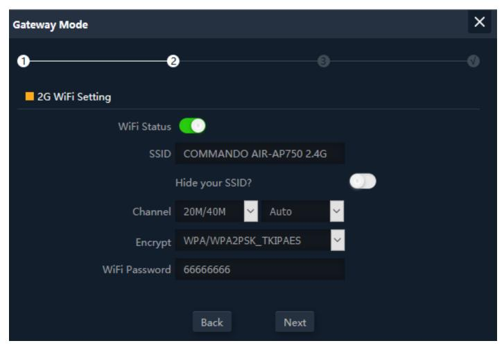
Fig 2.1.3 Gateway mode 2G Wi-Fi Setting of AirONE AP750
