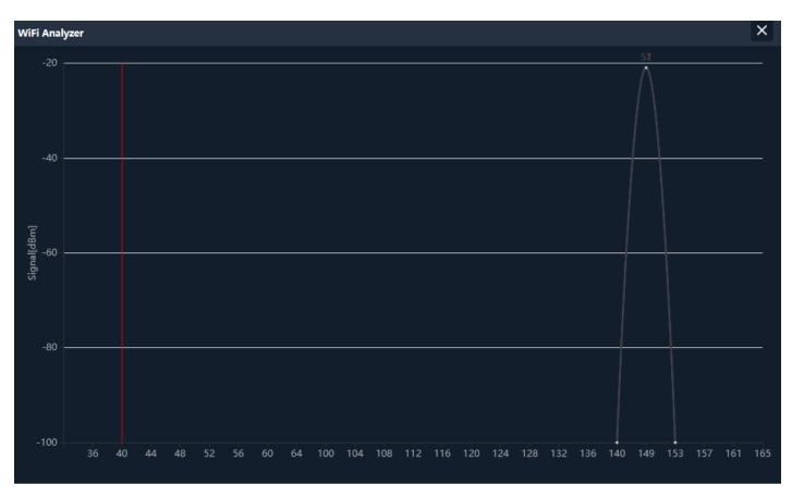
Fig 3.1.6 5G Wi-Fi Analyzer of AirONE AP750
