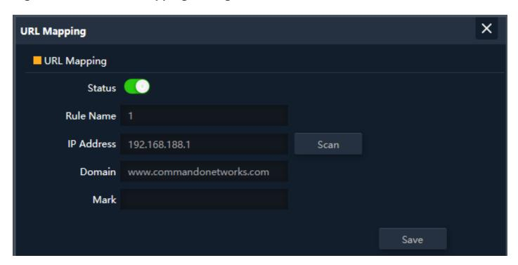
Fig 4.7.2 Configure URL Mapping setting for AirONE AP750
